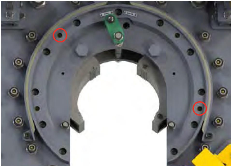
Illustration 3.E.1: Guide Ring Lubrication
