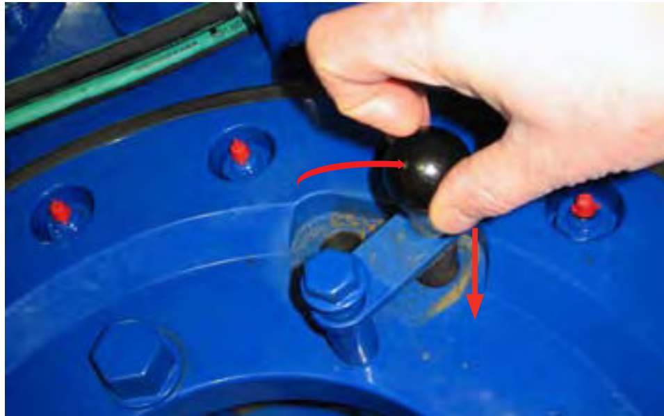
ILLUSTRATION 2.J.12: SETTING BACKING PIN TO BREAK-OUT POSITION
