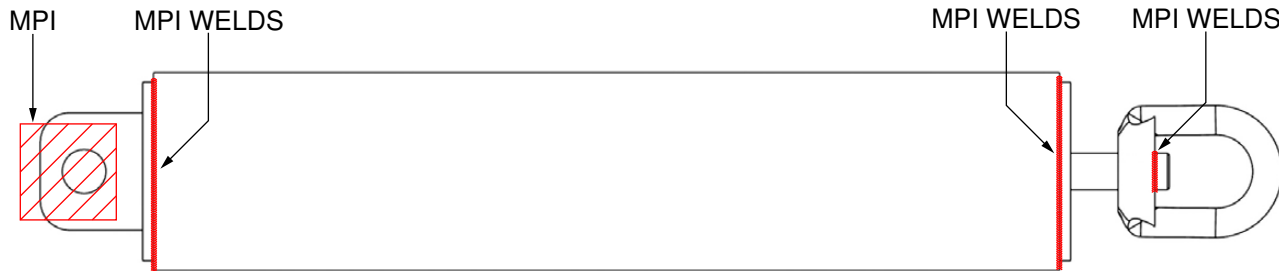
Illustration 5.7.1: Spring Hanger Inspection Area Map
