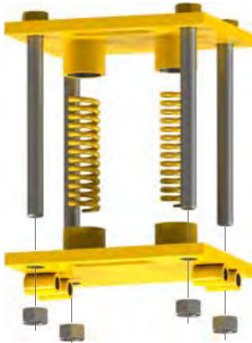
Illustration 5.9.12: Rear Leg Spring Support Installation (Model 80-0615-14)
