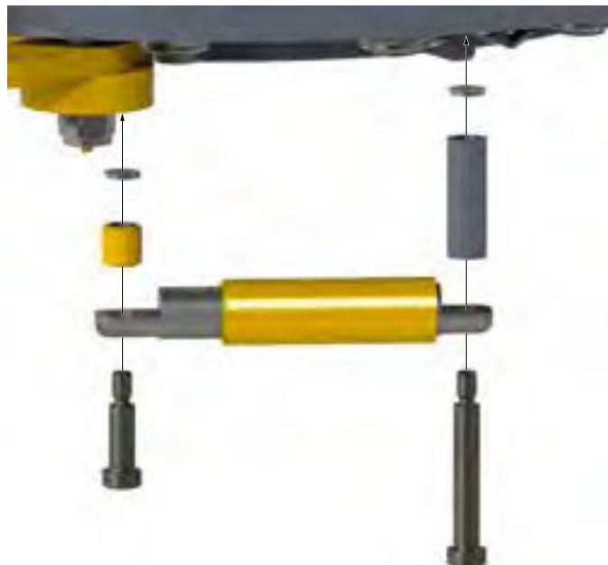
Illustration 5.9.10: Tong Assembly - Door Spring Stop Cylinder Installation
