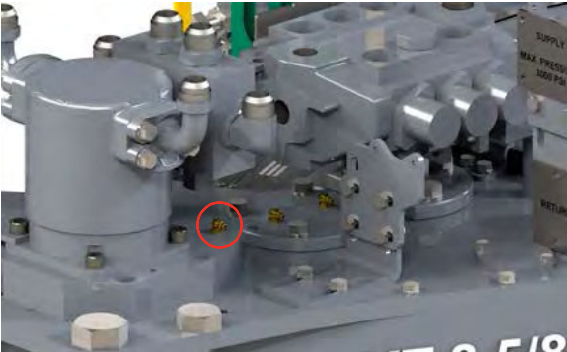
Illustration 5.5.7: Motor Mount Lubrication Point
