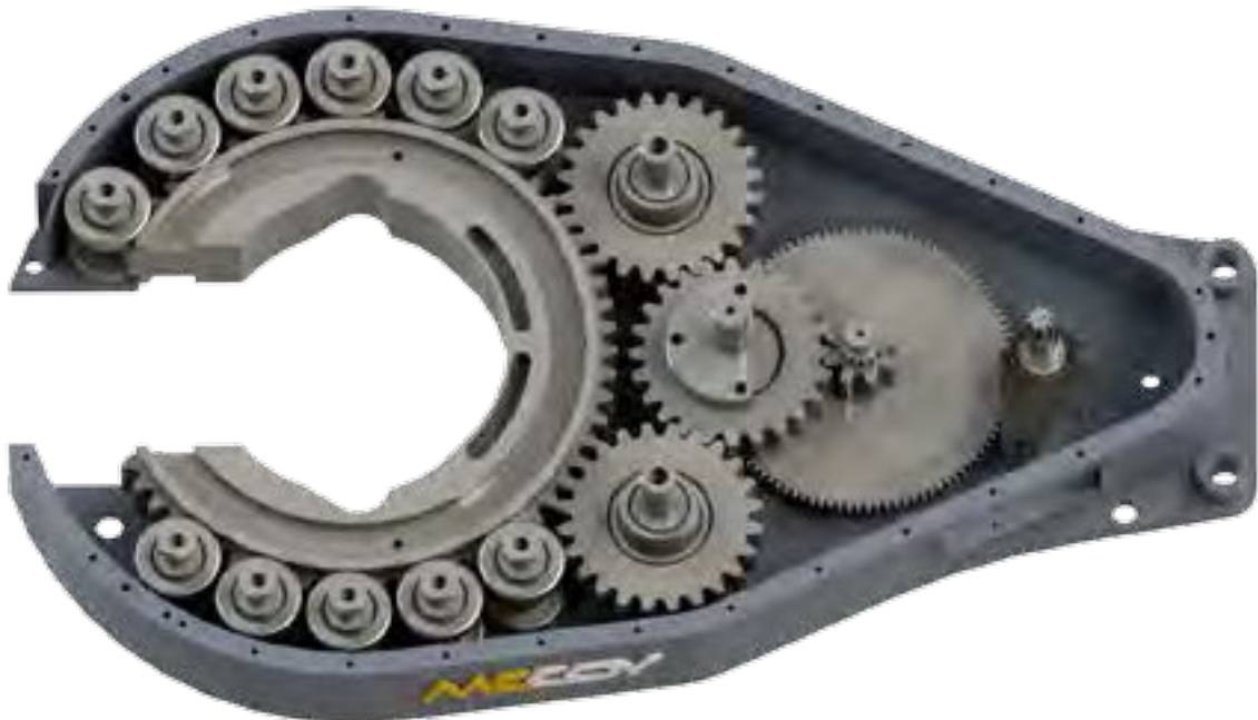
Illustration 5.9.2: Tong Assembly - Gear Assembly Positioning
