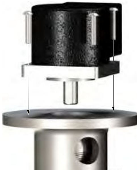
Illustration 8.1.3: Securing Encoder To Encoder Mount
