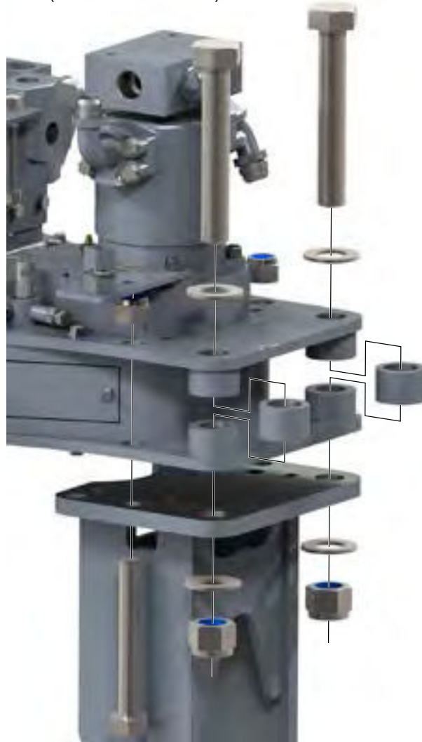
Illustration 5.9.13: Tong Assembly - Rear Leg Installation
