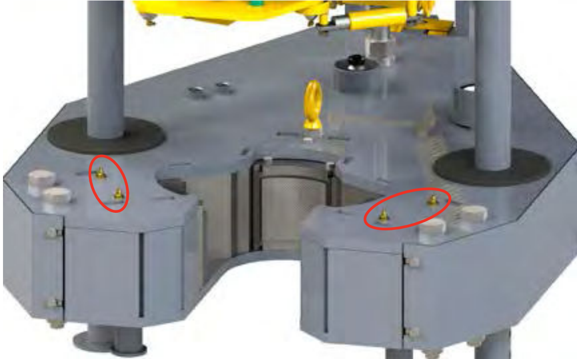
Illustration 5.5.12: CLINCHER® Cylinder Lubrication
