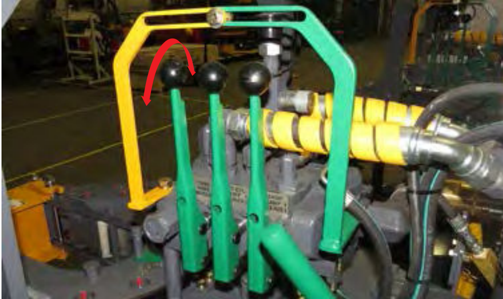
Illustration 4.0.1: Hydraulic Control - Tong Motor
