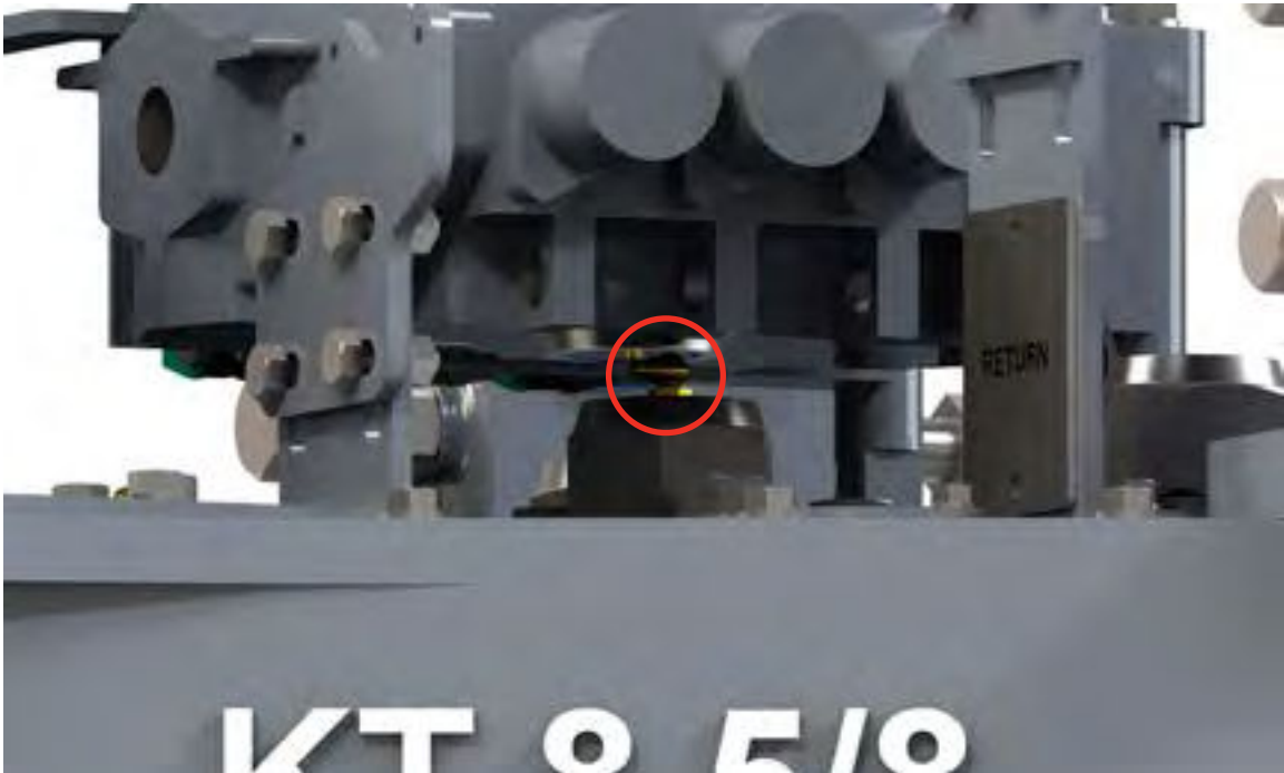
Illustration 5.5.4: Pinion Idler Lubrication Point
