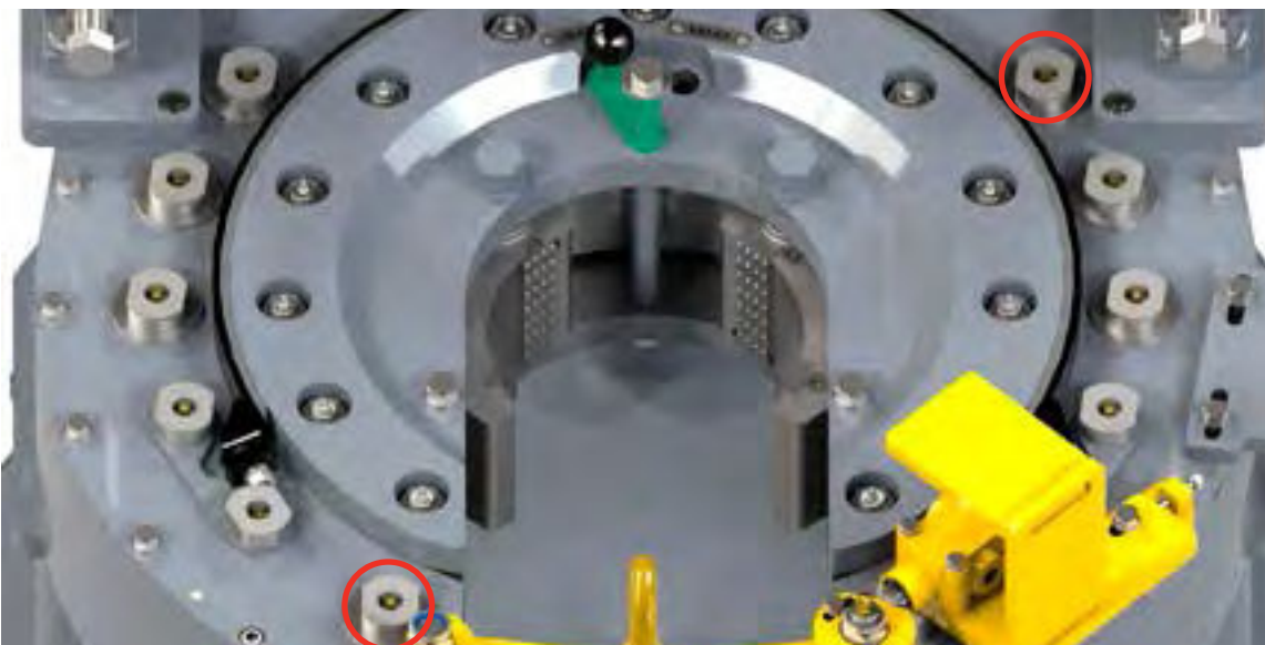
Illustration 5.5.2: Support Roller Lubrication
