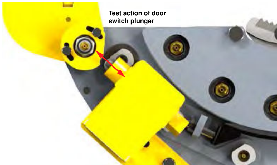
Illustration 5.6.4: Door Switch Adjustment 02
