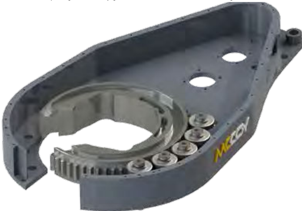
Illustration 5.9.1: Tong Assembly - Rotary Gear Installation
