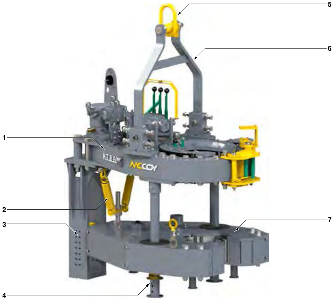
Illustration 2.1.1: KT8.625+CBU Component Identification 01 (Model 80-0615-10 Shown)
