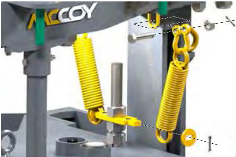
Illustration 5.9.16: Rear Backup Support Spring Installation (Tension LC-Style Backups)
