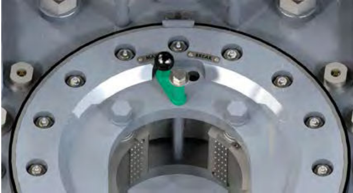
Illustration 4.1.2: Setting Backing Pin To “Make-up” Position
