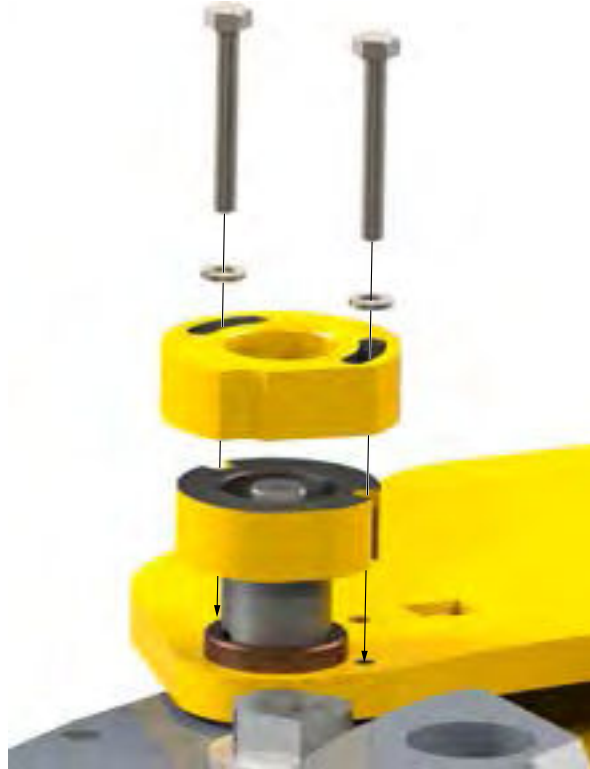
Illustration 5.9.9: Tong Assembly - Door Switch Cam Installation
