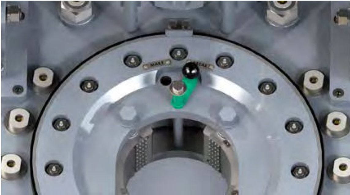
Illustration 4.1.3: Backing Pin Set To “Break-Out” Position
