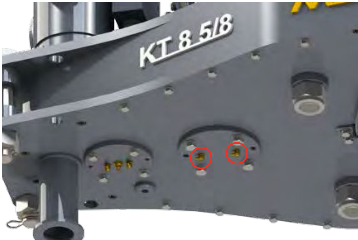
Illustration 5.5.5: Pinion Bearing Lubrication Points
