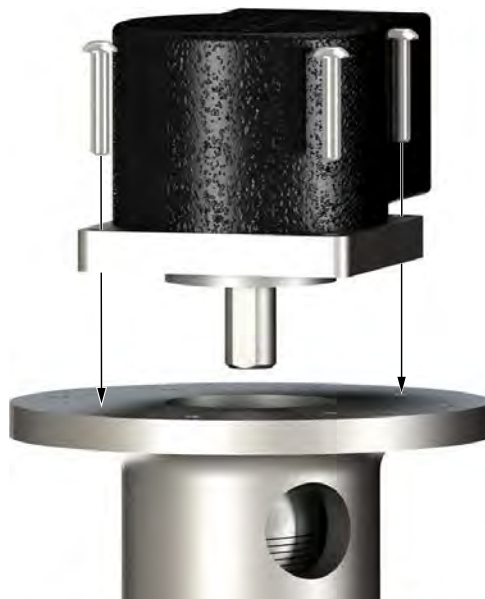
Illustration 8.1.3: Securing Encoder To Encoder Mount
