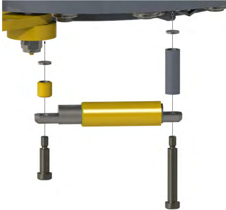
Illustration 5.9.9: Tong Assembly - Door Spring Stop Cylinder Installation
