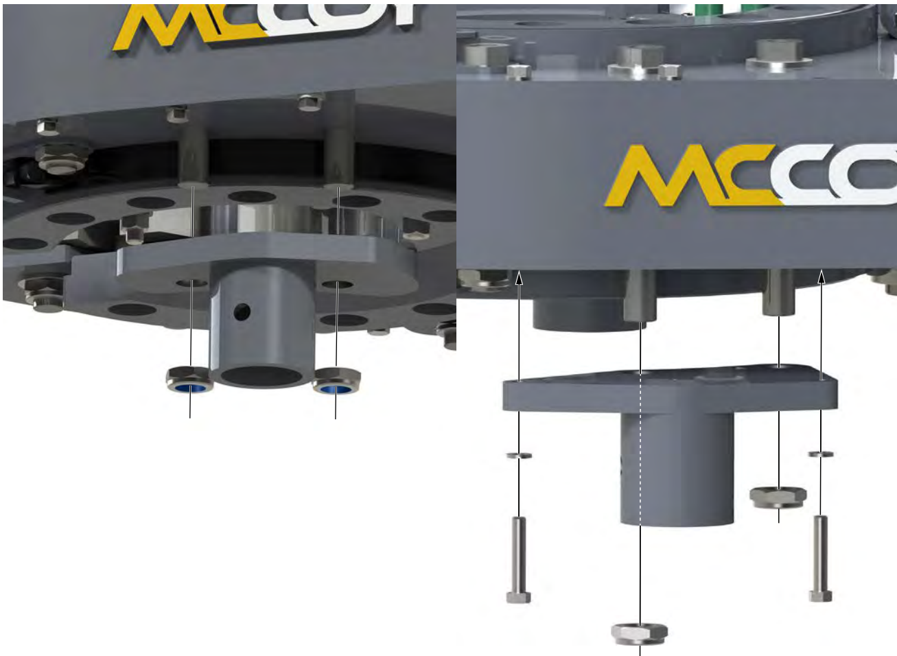
Illustration 5.9.7: Tong Assembly - Front Leg Mount Weldment Installation
