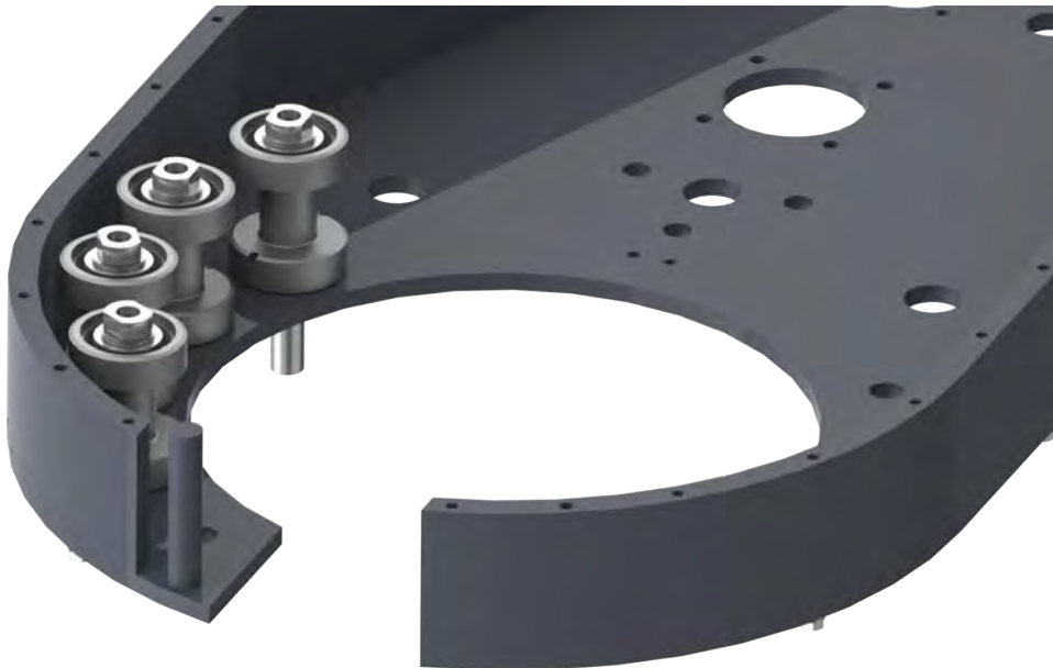
Illustration 5.9.1: Tong Assembly - Initial Support Roller Installation
