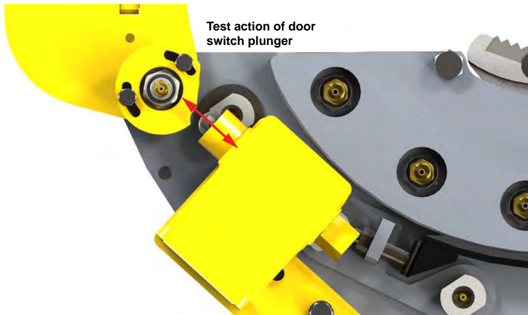
Illustration 5.6.4: Door Switch Adjustment 02
