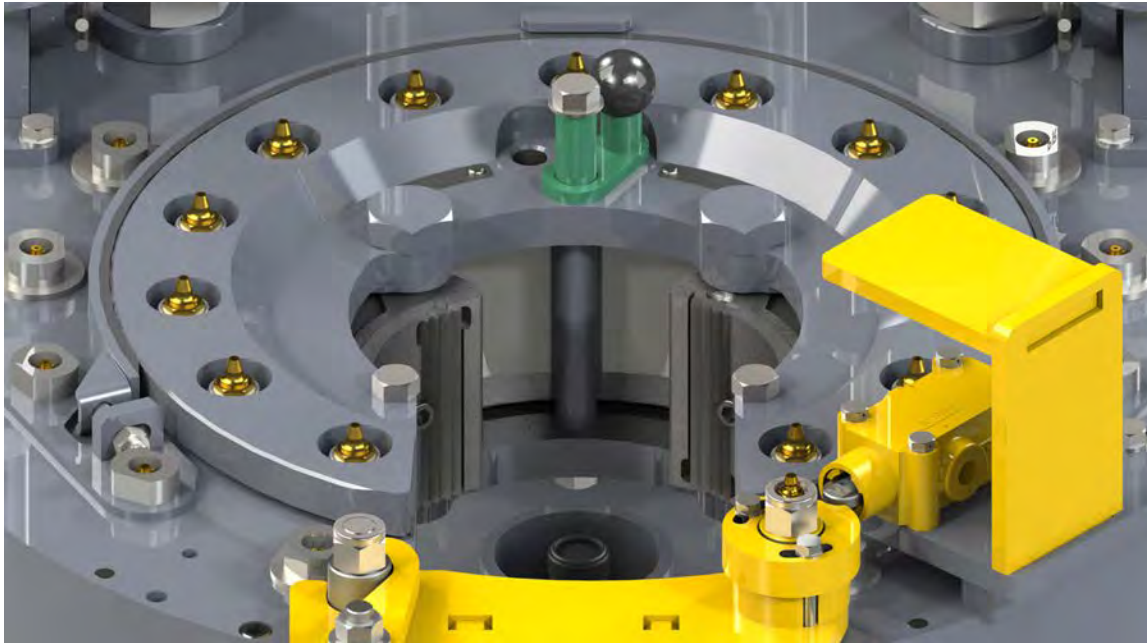
Illustration 4.1.3: Backing Pin Set To “Break-Out” Position
