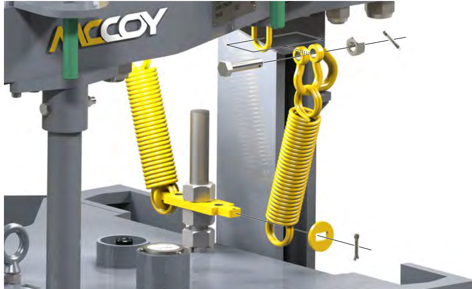
Illustration 5.9.14: Rear Backup Support Spring Installation (Tension LC-Style Backups)
