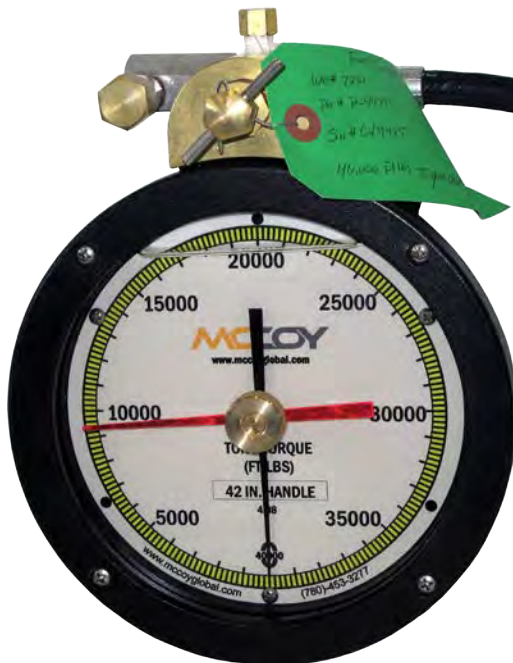
Illustration 8.0.1: Torque Gauge (For Illustration Purposes Only)
