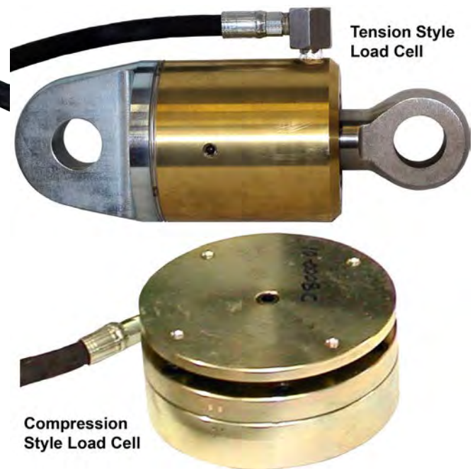
Illustration 8.0.2: Load Cell Types
