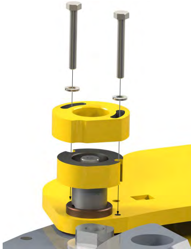
Illustration 5.9.8: Tong Assembly - Door Switch Cam Installation
