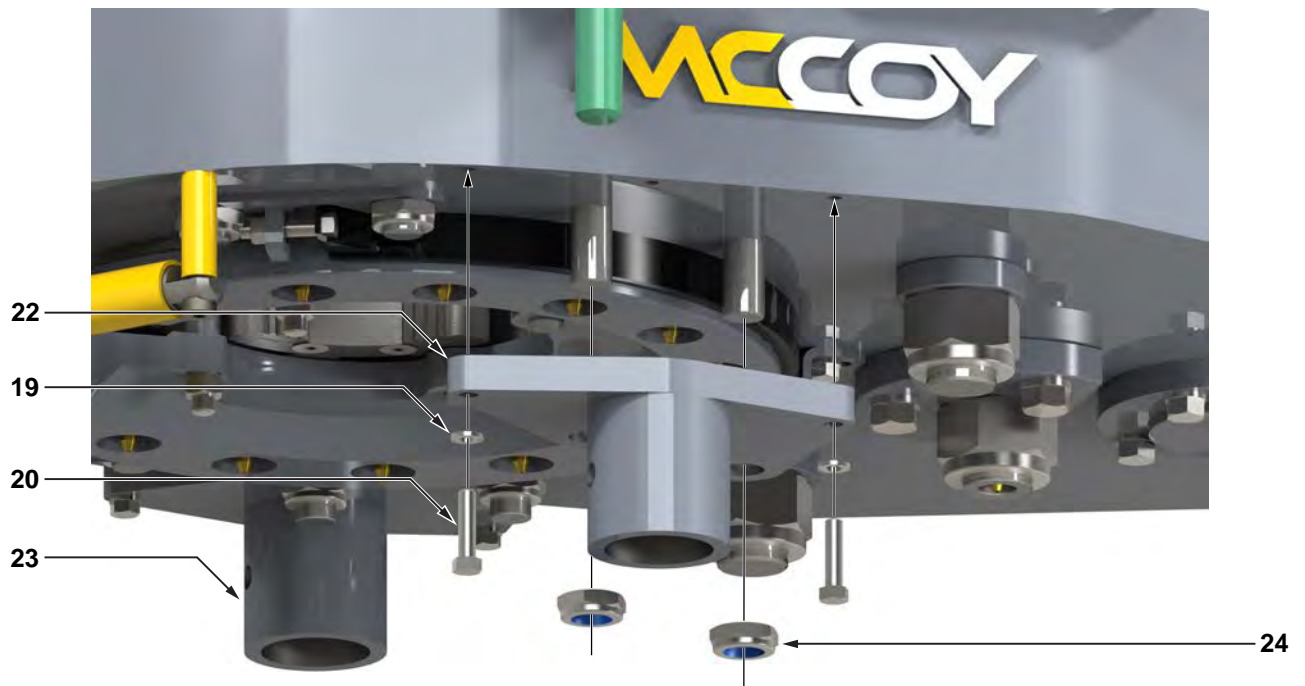
Illustration 7.38: 80-0421-10 KT5.5+CBUT Front Leg Mounts
