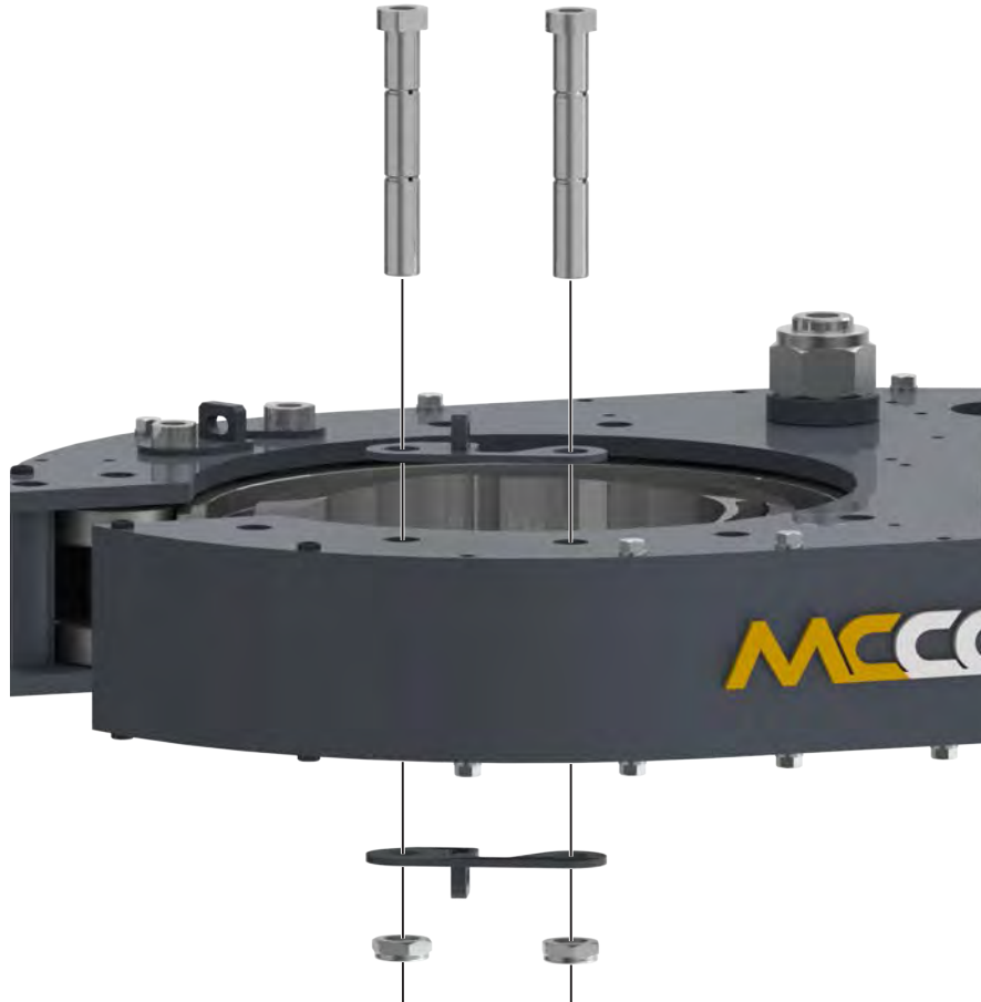
Illustration 5.9.6: Tong Assembly - Brake Band Lug Weldment Installation
