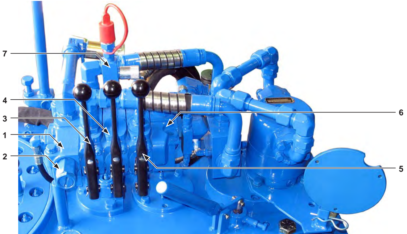
Illustration 3.3.2: KT5.5+CBU Hydraulic Component ID 01
