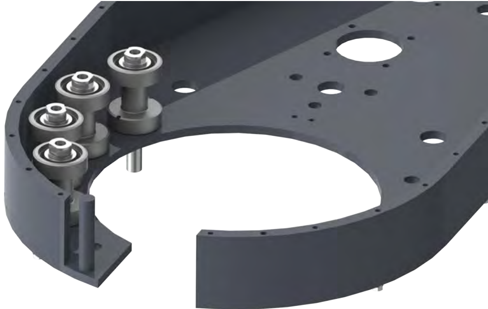
ILLUSTRATION 4.I.1: TONG ASSEMBLY - INITIAL SUPPORT ROLLER INSTALLATION
