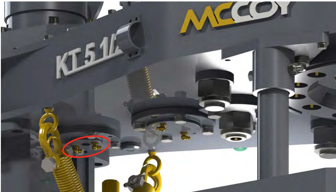
ILLUSTRATION 4.E.7: CLUTCH BEARING LUBRICATION
