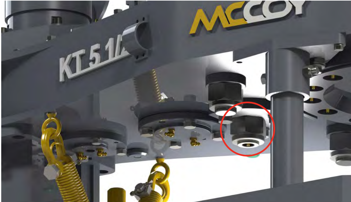
ILLUSTRATION 3.D.4: PINION IDLER BEARING LUBRICATION
