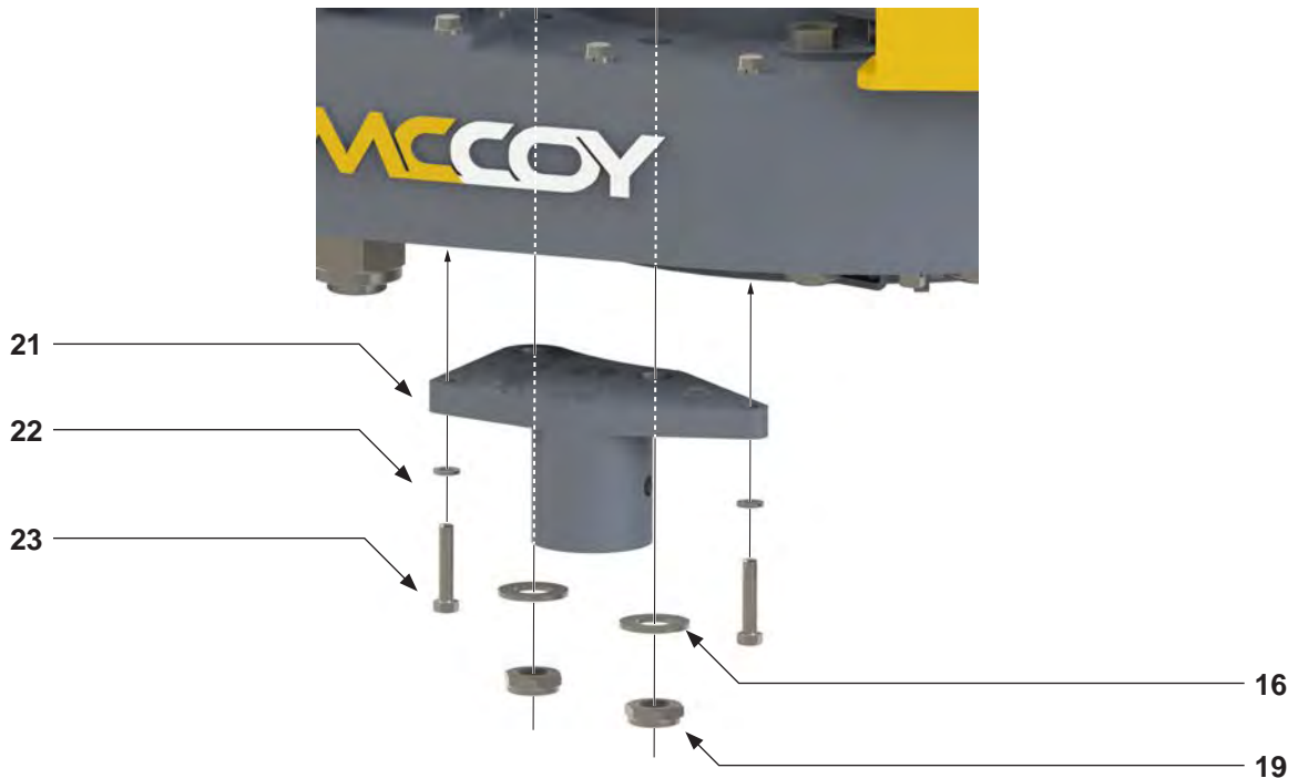
ILLUSTRATION 6.39: FRONT LEG WELDMENT INSTALLATION
