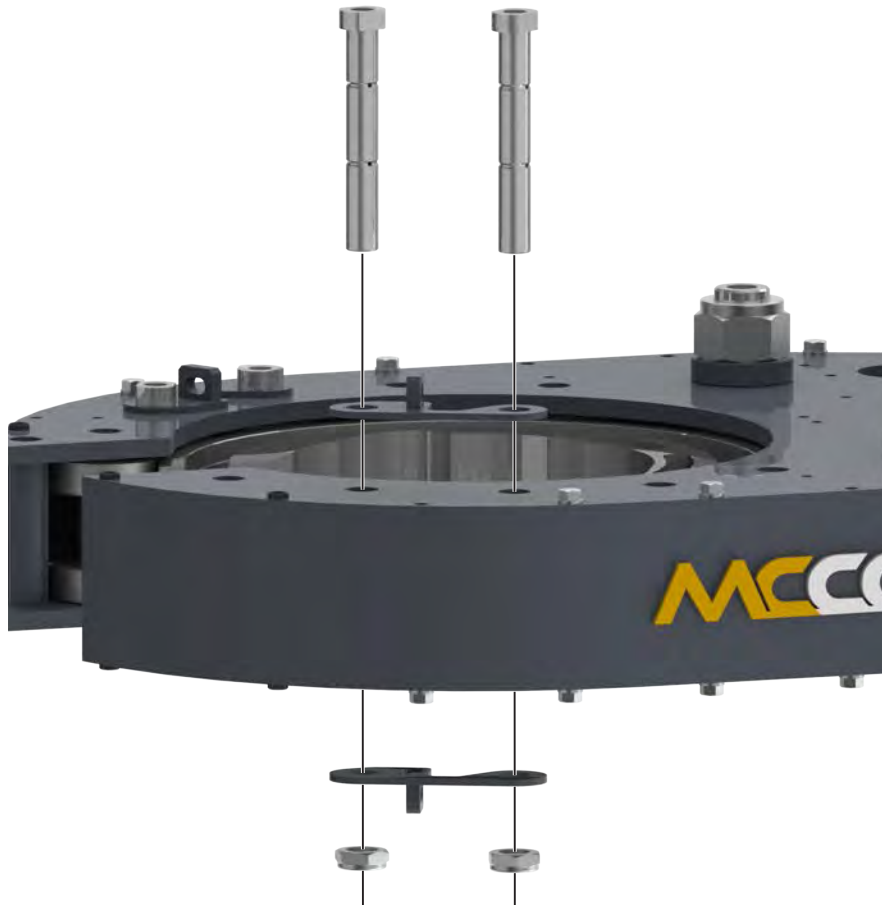
ILLUSTRATION 4.I.5: TONG ASSEMBLY - BRAKE BAND WELDMENT INSTALLATION
