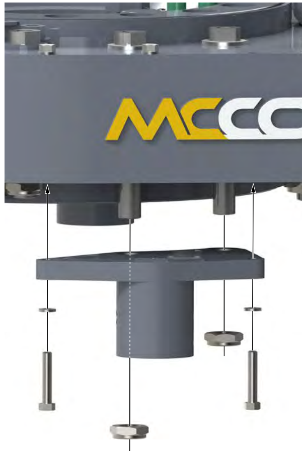
ILLUSTRATION 4.1.6: TONG ASSEMBLY - FRONT LEG MOUNT WELDMENT INSTALLATION
