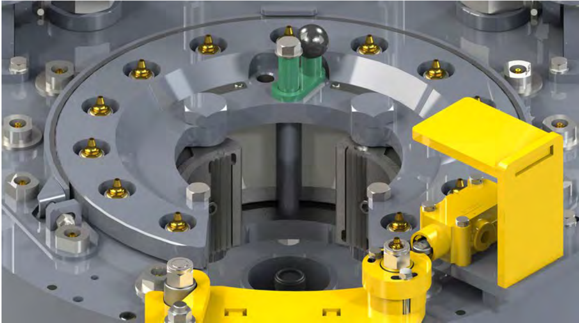
ILLUSTRATION 3.B.4: BACKING PIN CONFIGURED FOR "MAKE-UP" OPERATIONS
