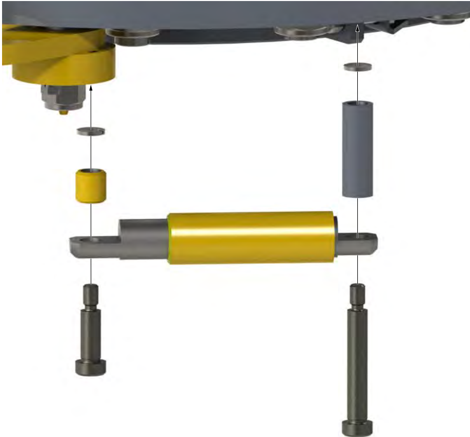
ILLUSTRATION 4.I.11: TONG ASSEMBLY - DOOR STOP SPRING CYLINDER INSTALLATION
