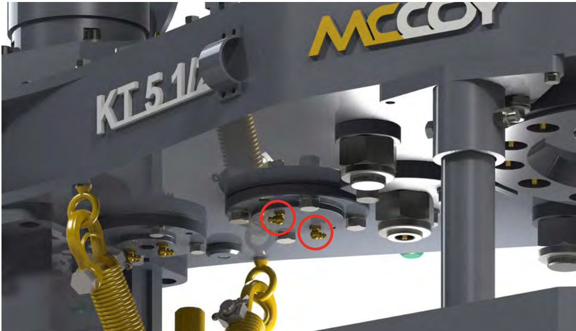
ILLUSTRATION 4.E.6: PINION BEARING LUBRICATION (BOTTOM)
