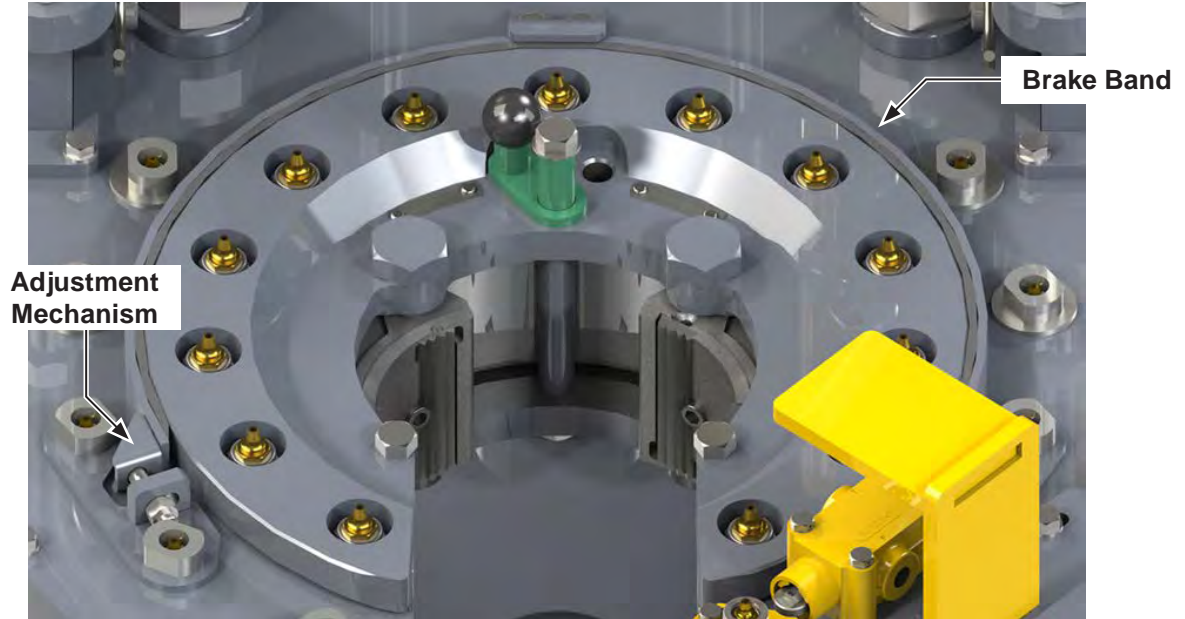
ILLUSTRATION 4.F.1: BRAKE BAND ADJUSTMENT
