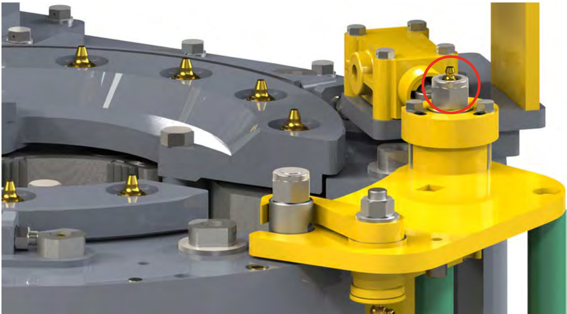
ILLUSTRATION 4.E.11: DOOR PIVOT BUSHING LUBRICATION
