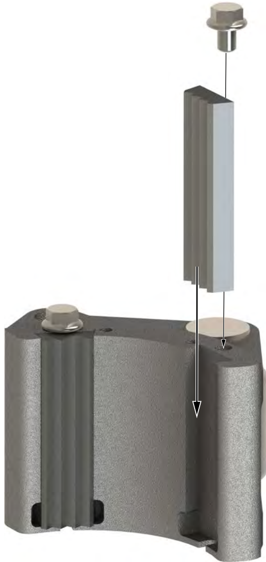
ILLUSTRATION 2.F.2: KT5500 STANDARD JAW DIE REMOVAL
