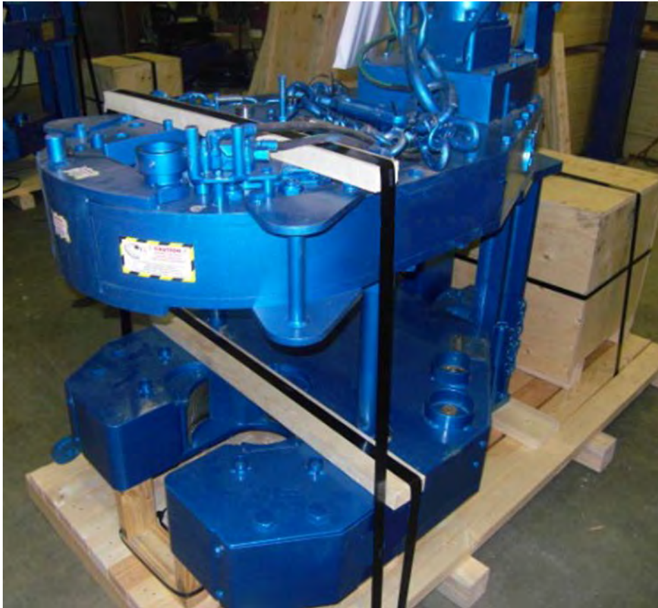
ILLUSTRATION 4.M.4: SHIPPING INSTRUCTIONS - STRAPPING EQUIPMENT TO PALLET
