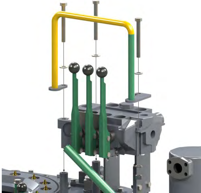
ILLUSTRATION 4.1.12: TONG ASSEMBLY - VALVE ASSEMBLY INSTALLATION
