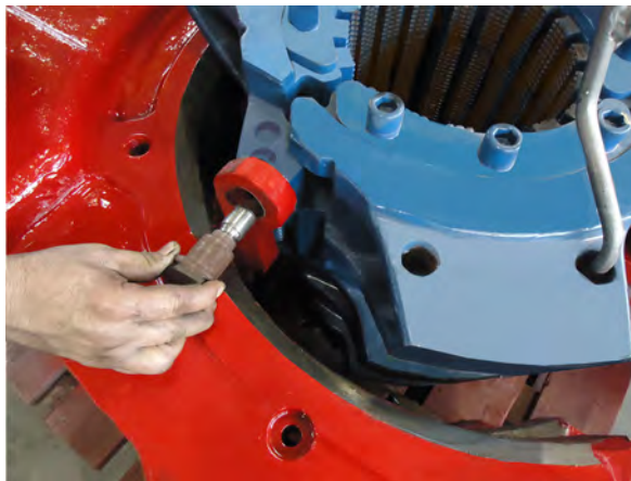
Figure 5: Slip Change – removing retainer pin
