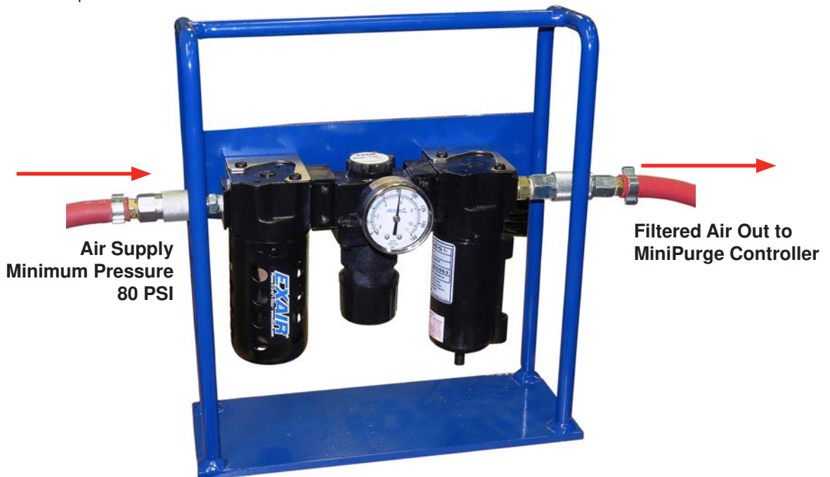
Illustration 3.1.11: WINCATT® Ex Purge Air Filter Assembly
