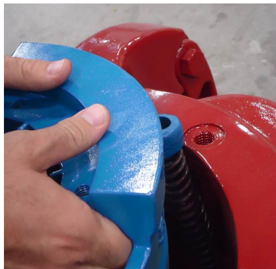
Figure 3 – Compressing spring to install slip
