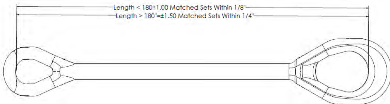
Figure 4: Link contact length
