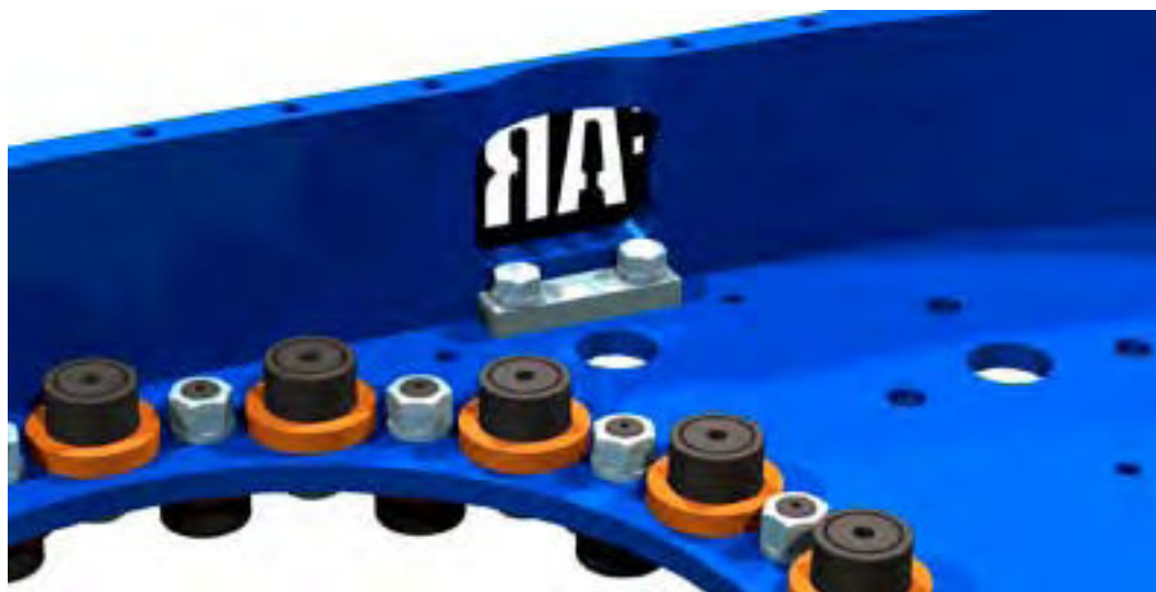
ILLUSTRATION 3.H.2: IDLER SHAFT RESTRAINT BLOCK INSTALLATION
