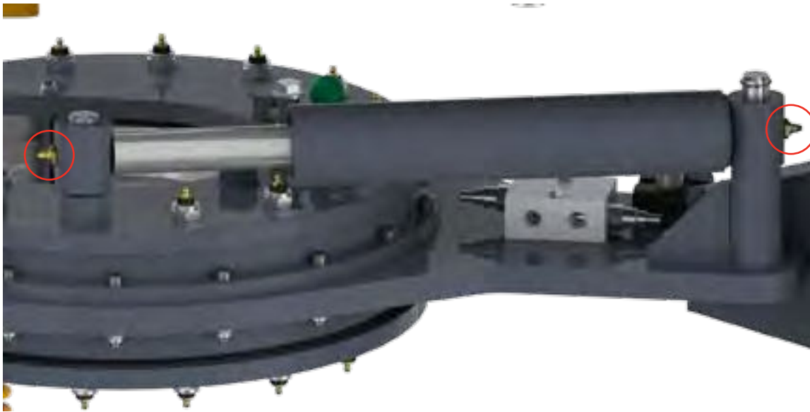
ILLUSTRATION 3.D.13: BACKUP CLAMP CYLINDER LUBRICATION
