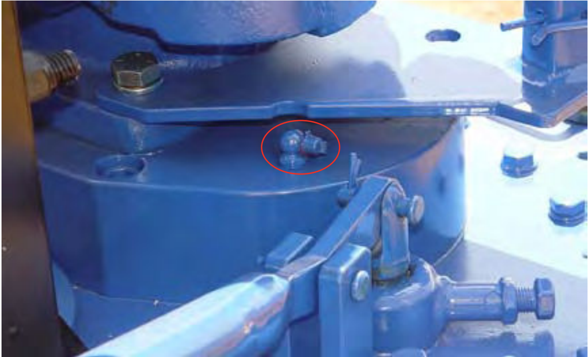
ILLUSTRATION 3.D.7: MOTOR MOUNT LUBRICATION
