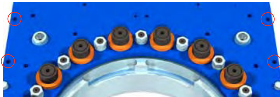
ILLUSTRATION 3.H.6: RIGID SLING BRACKET INSTALLATION LOCATIONS
