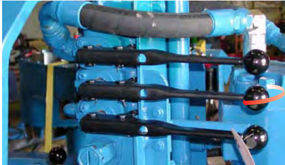
ILLUSTRATION 2.H.13: LOWERING TONG & BACKUP USING LIFT CYLINDER CONTROL
