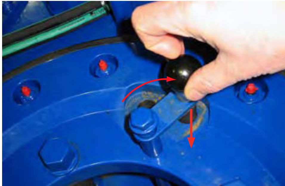
ILLUSTRATION 2.H.10: SETTING BACKING PIN TO "BREAK-OUT" POSITION
