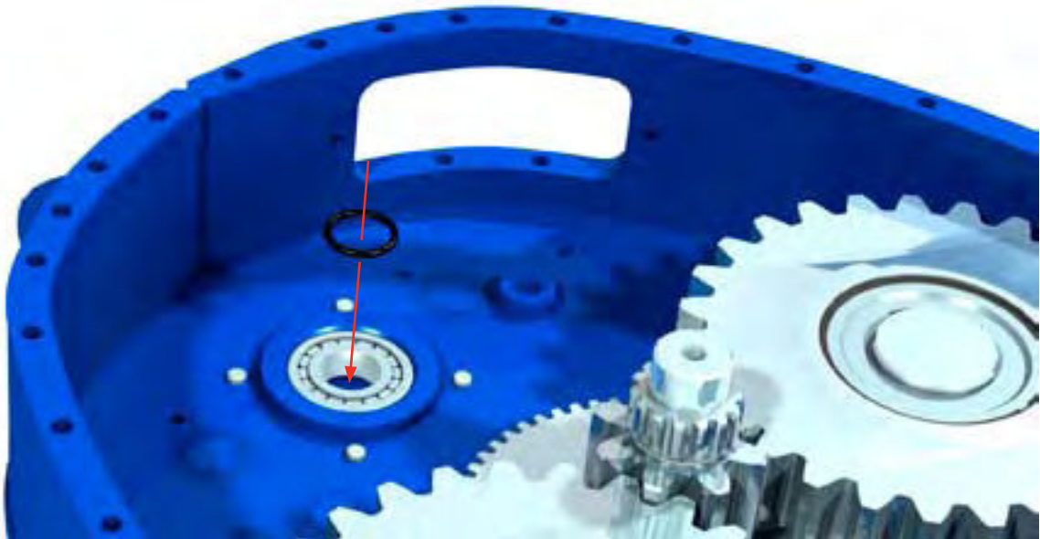
ILLUSTRATION 3.H.4: CLUTCH O-RING INSTALLATION
