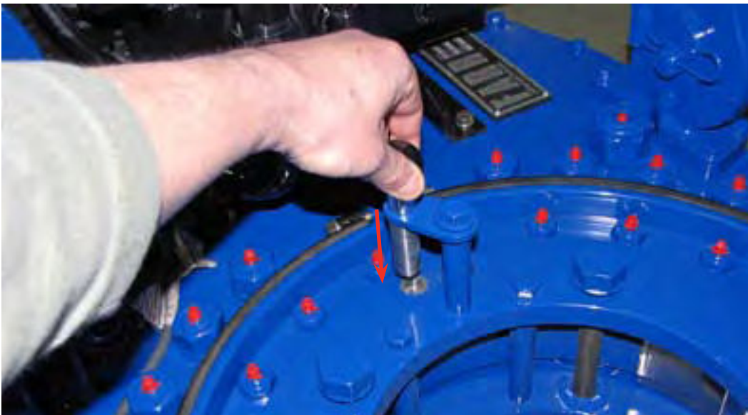
ILLUSTRATION 2.H.2: SETTING BACKING PIN TO “MAKE-UP” POSITION
