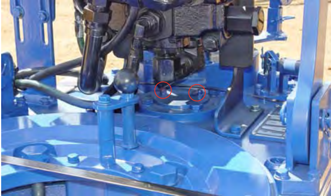
ILLUSTRATION 3.D.4: PINION LUBRICATION (TOP PLATE)
