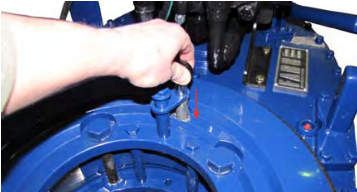
ILLUSTRATION 2.H.8: SETTING BACKING PIN TO "BREAK-OUT" POSITION
