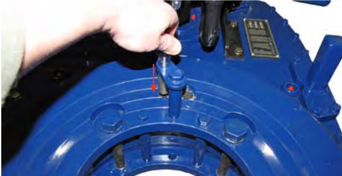
ILLUSTRATION 2.H.2: SETTING BACKING PIN TO "MAKE-UP" POSITION
