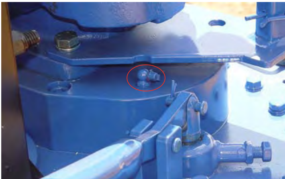
ILLUSTRATION 3.D.7: MOTOR MOUNT LUBRICATION
