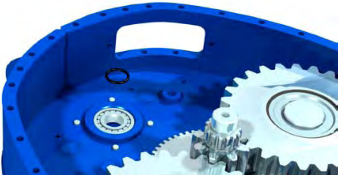
ILLUSTRATION 3.H.4: CLUTCH O-RING INSTALLATION
