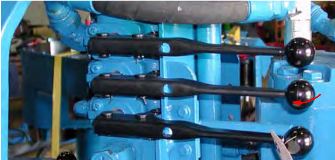
ILLUSTRATION 2.H.11: LOWERING TONG USING LIFT CYLINDER CONTROL
