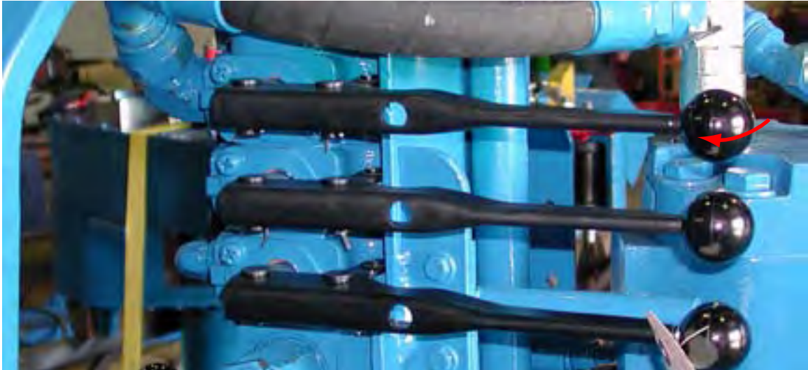
ILLUSTRATION 2.H.6: MOTOR CONTROL - RELEASING JAWS
