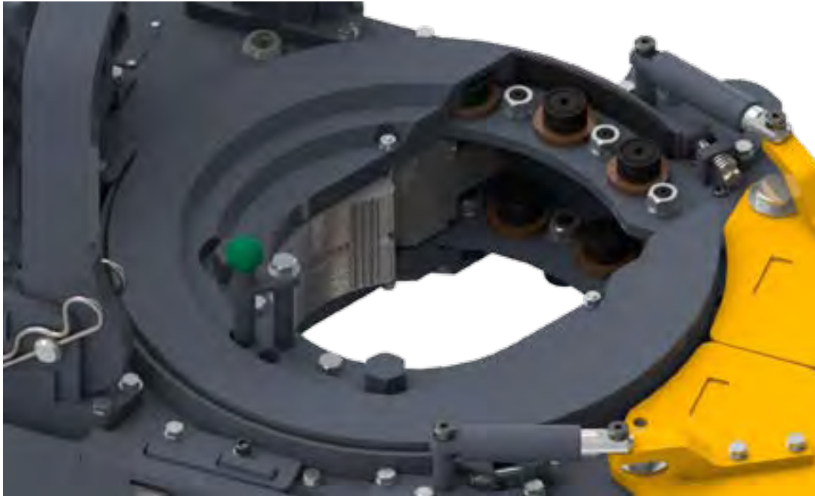
ILLUSTRATION 3.D.1: CAGE PLATE / CAM FOLLOWER LUBRICATION
