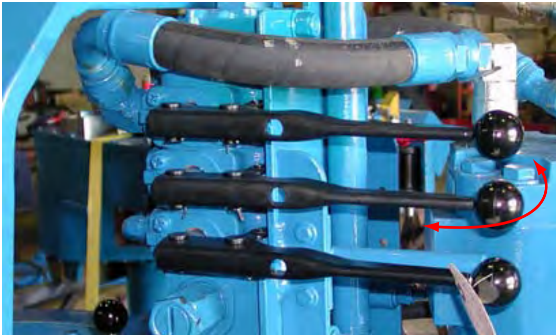
ILLUSTRATION 2.G.2: TONG LIFT CYLINDER VALVE
