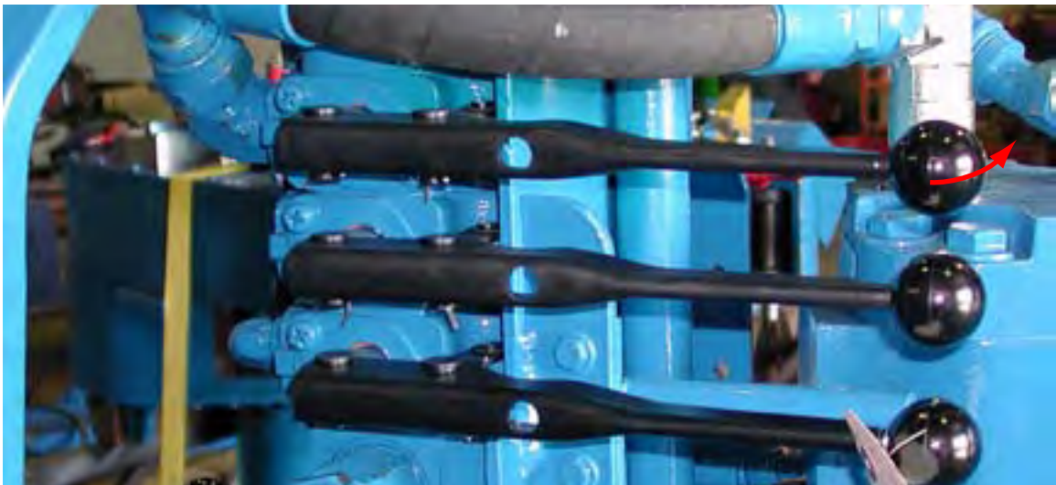
ILLUSTRATION 2.H.10: RELEASING TONG JAWS FOLLOWING BREAK-OUT & UN-THREADING
