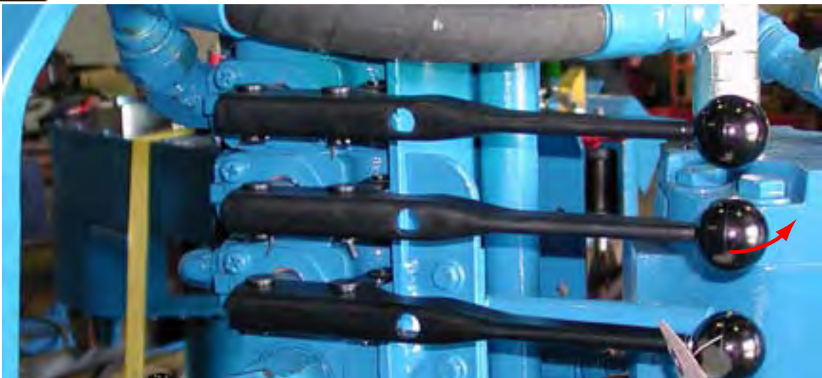
ILLUSTRATION 2.H.3: LIFT CYLINDER CONTROL - RAISE
