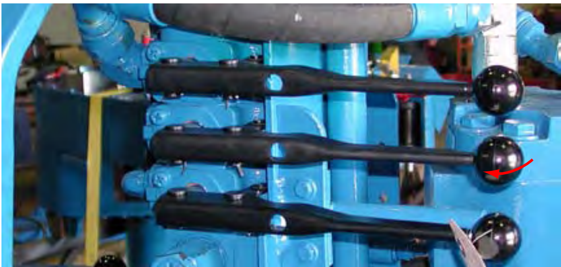
ILLUSTRATION 2.H.7: LIFT CYLINDER CONTROL - LOWER
