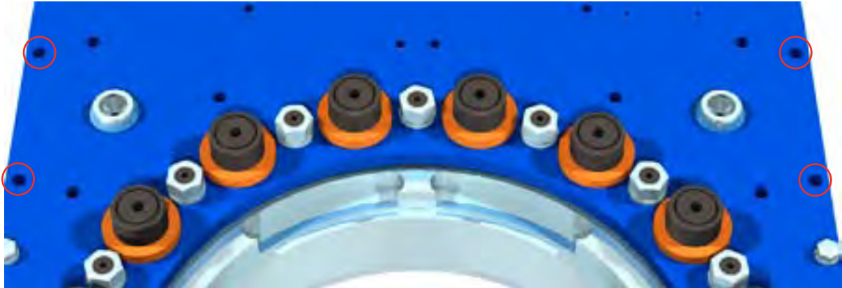
ILLUSTRATION 3.H.6: RIGID SLING BRACKET INSTALLATION LOCATIONS
