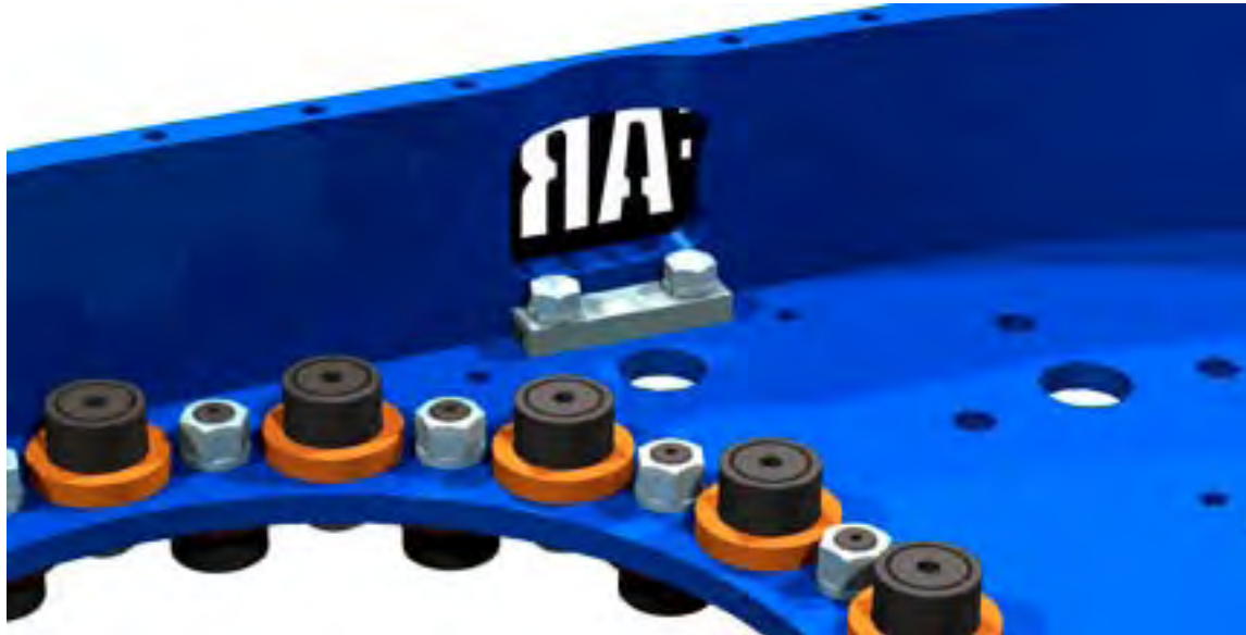
ILLUSTRATION 3.H.2: IDLER SHAFT RESTRAINT BLOCK INSTALLATION
