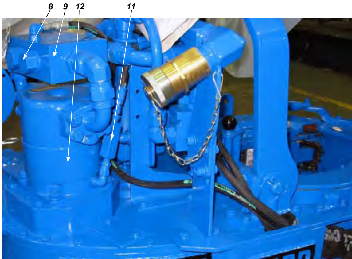
ILLUSTRATION 2.C.3: LW9625 HYDRAULIC COMPONENT IDENTIFICATION 02
