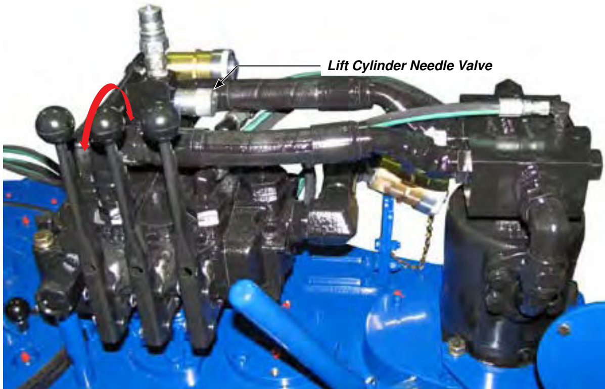
ILLUSTRATION 2.1.2: HYDRAULIC CONTROL - LIFT CYLINDER
