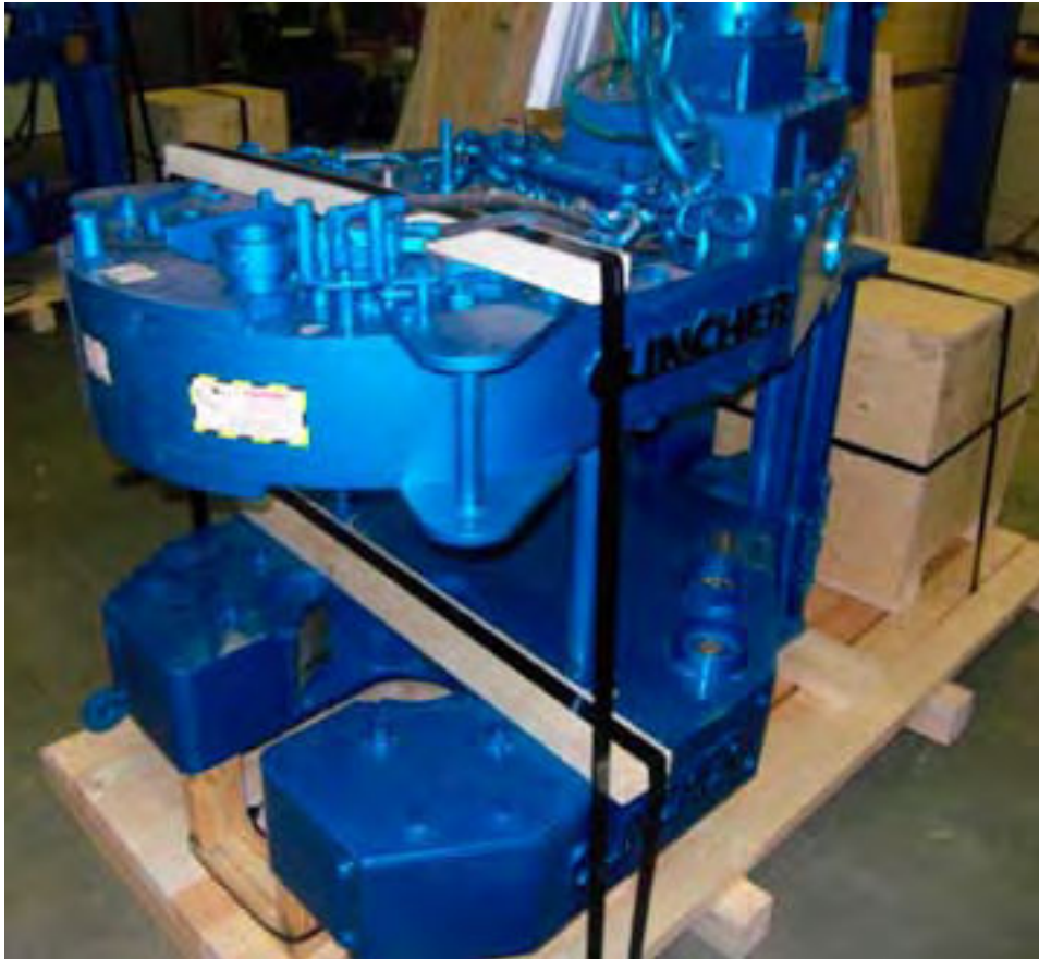
ILLUSTRATION 3.M.4: SHIPPING INSTRUCTIONS - STRAPPING EQUIPMENT TO PALLET
