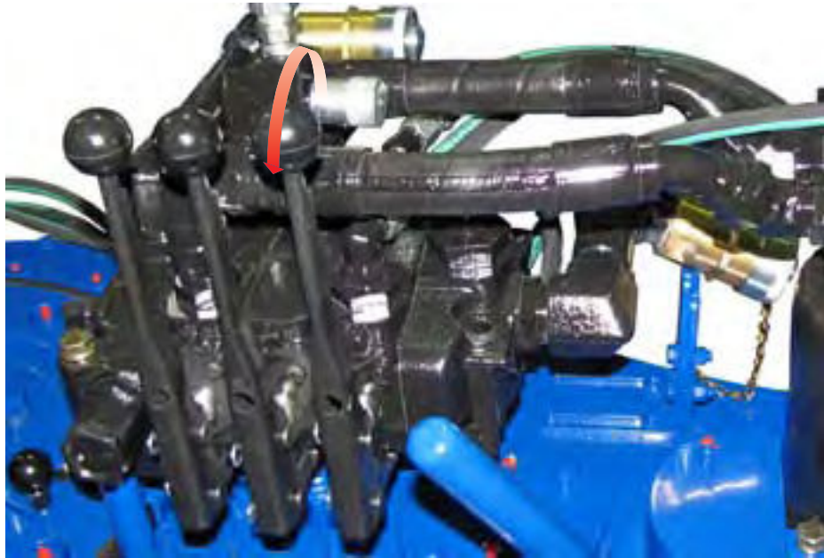
ILLUSTRATION 2.J.8: USING BACKUP CONTROL TO RELEASE BACKUP JAWS
