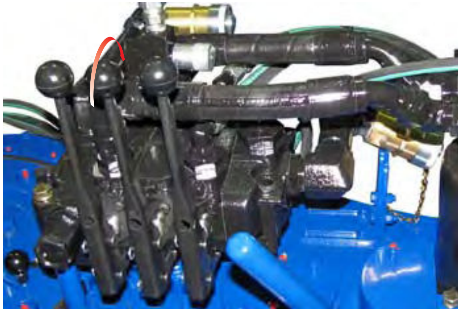
ILLUSTRATION 2.J.9: USING LIFT CYLINDER CONTROL TO LOWER ASSEMBLY
