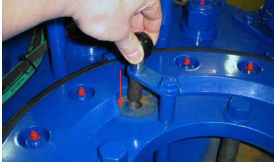
ILLUSTRATION 2.J.2: SETTING BACKING PIN TO “MAKE-UP” POSITION
