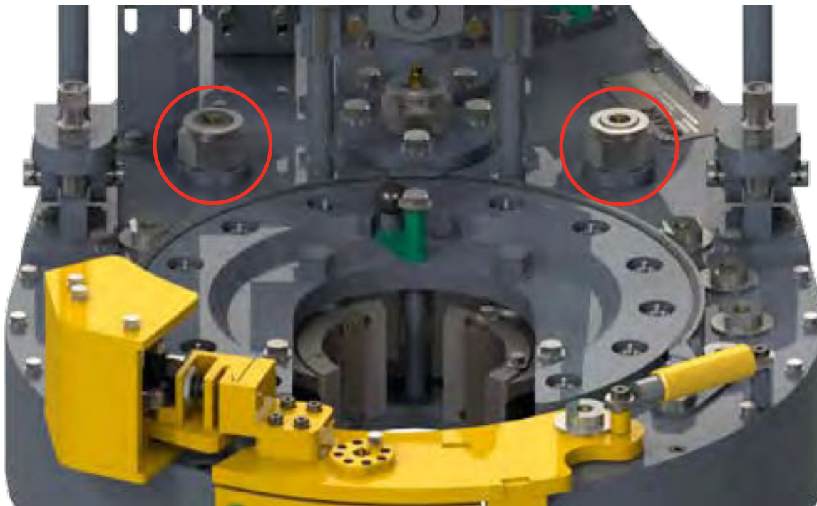
ILLUSTRATION 3.E.3: ROTARY IDLER LUBRICATION
