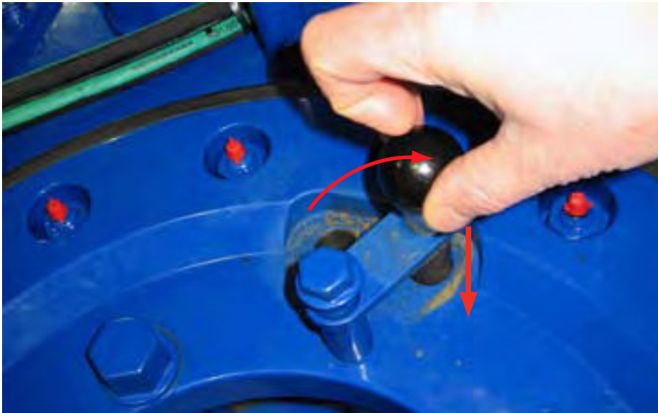
ILLUSTRATION 2.J.10: SETTING BACKING PIN TO BREAK-OUT POSITION
