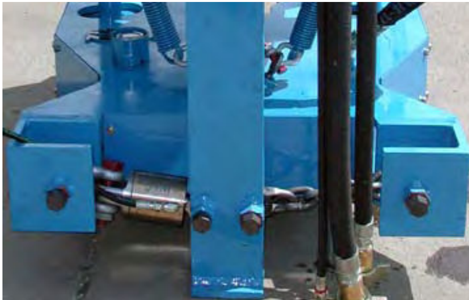
ILLUSTRATION 2.H.5: TENSION LOAD CELL CONFIGURATION - MAKE UP
