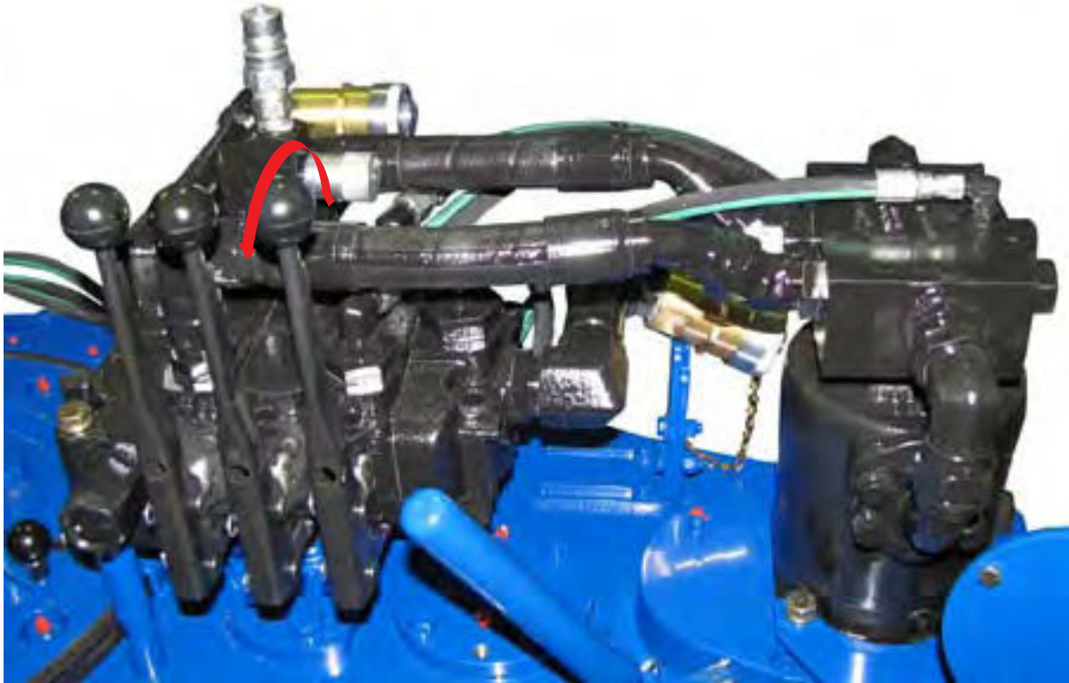
ILLUSTRATION 2.1.3: HYDRAULIC CONTROL - BACKUP
