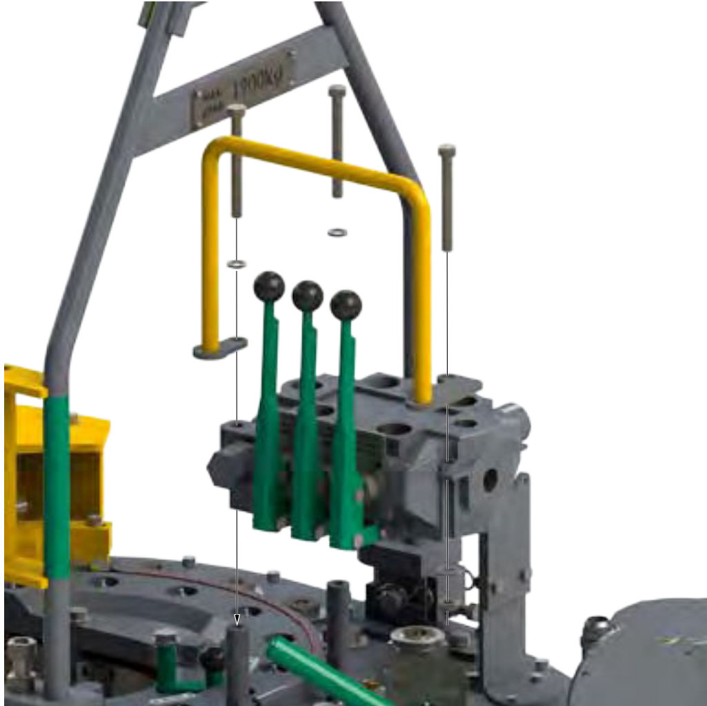
ILLUSTRATION 3.I.11: TONG ASSEMBLY - VALVE HANDLE GUARD INSTALLATION (CE MARKED)
