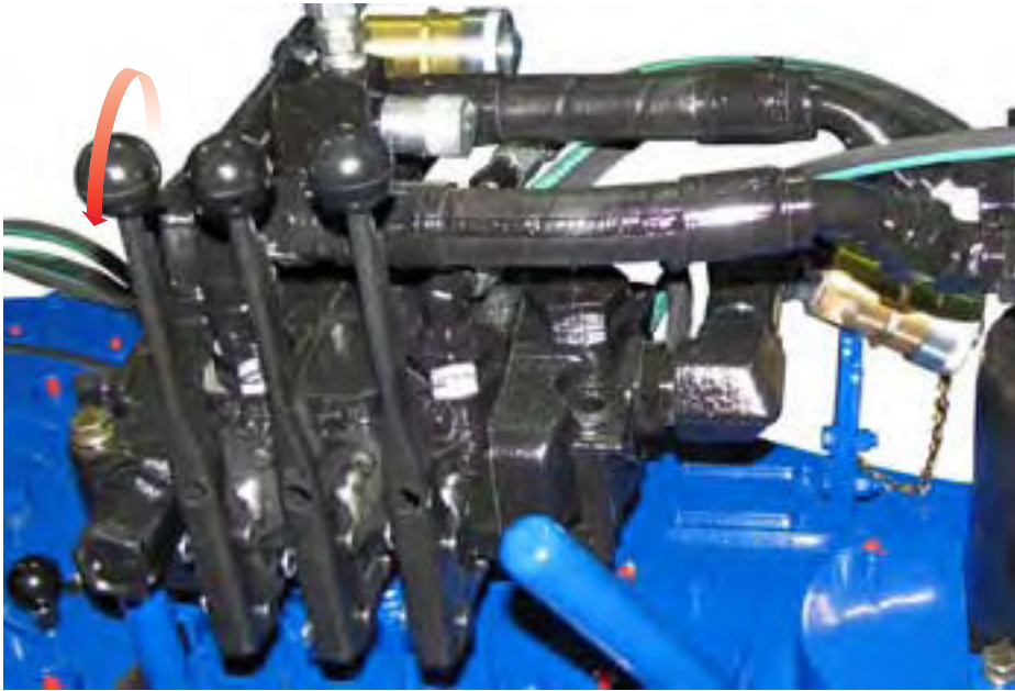
ILLUSTRATION 2.J.7: USING MOTOR CONTROL TO RELEASE JAWS IN “MAKE UP” MODE
