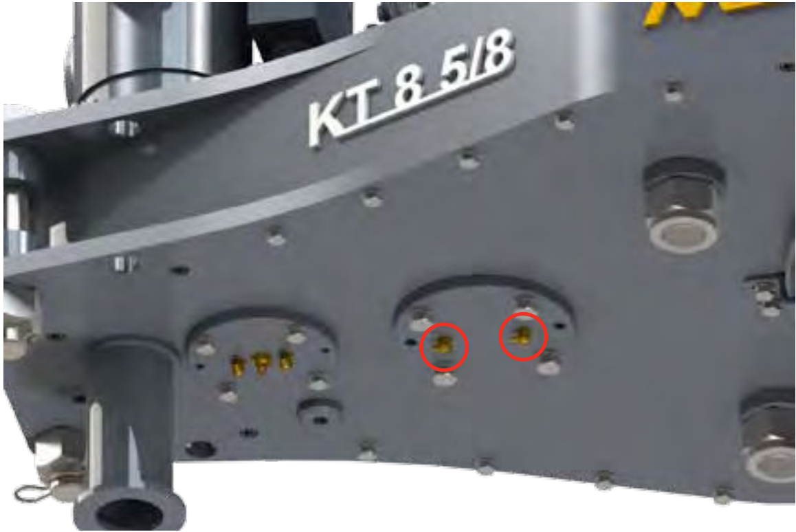
ILLUSTRATION 3.E.6: PINION LUBRICATION POINTS (BOTTOM PLATE)
