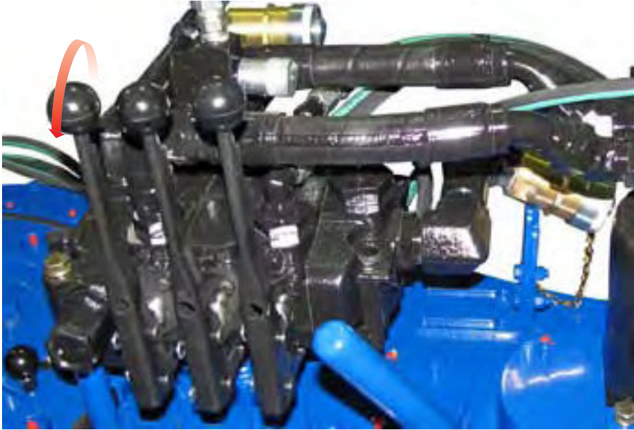
ILLUSTRATION 2.J.12: USING MOTOR CONTROL TO RELEASE JAWS IN “BREAK OUT” MODE
