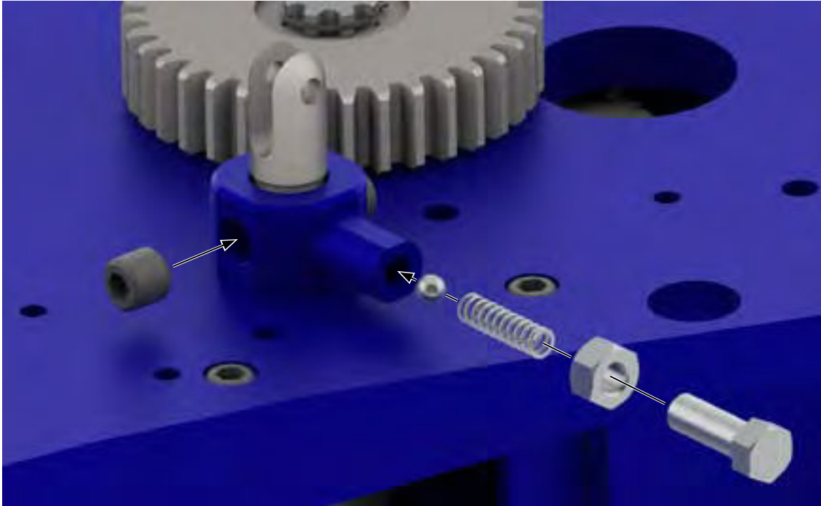
ILLUSTRATION 3.1.7: TONG ASSEMBLY - TOP SHIFTER BUSHING ASSEMBLY
