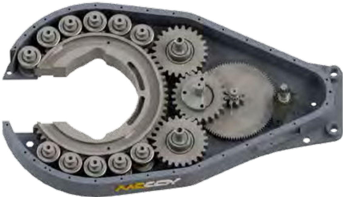
ILLUSTRATION 3.1.2: TONG ASSEMBLY - GEAR ASSEMBLY POSITIONING
