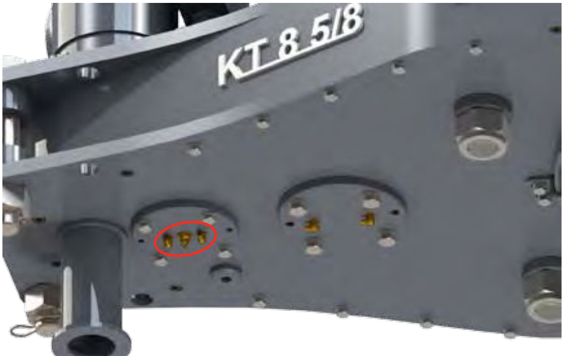
ILLUSTRATION 3.E.7: CLUTCH LUBRICATION POINTS
