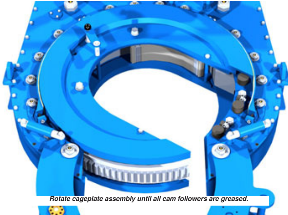
ILLUSTRATION 3.D.1: CAGEPLATE CAM FOLLOWER LUBRICATION
