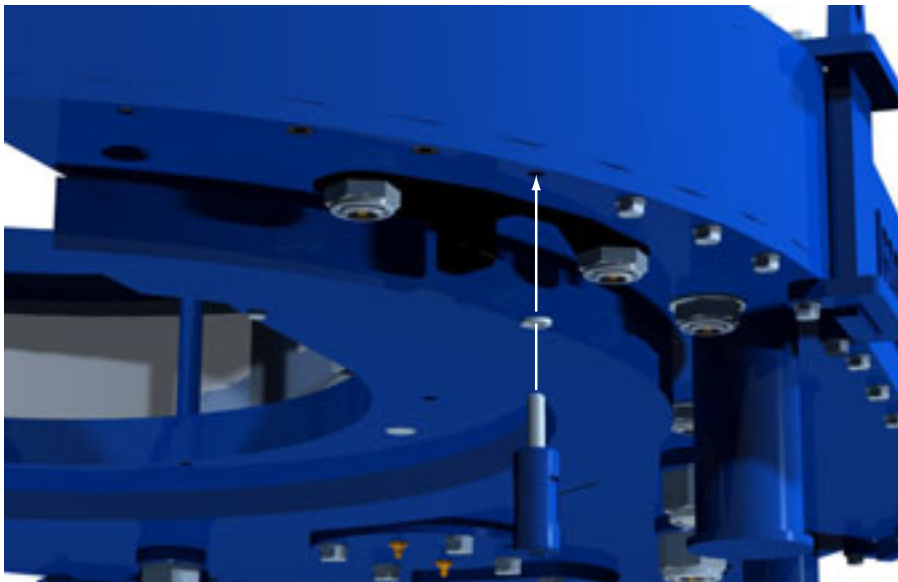
ILLUSTRATION 3.H.10: DOOR CYLINDER POST INSTALLATION
