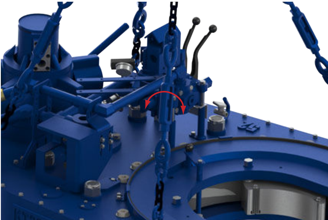
ILLUSTRATION 2.F.3: LEVELING TONG USING TURNBUCKLES
