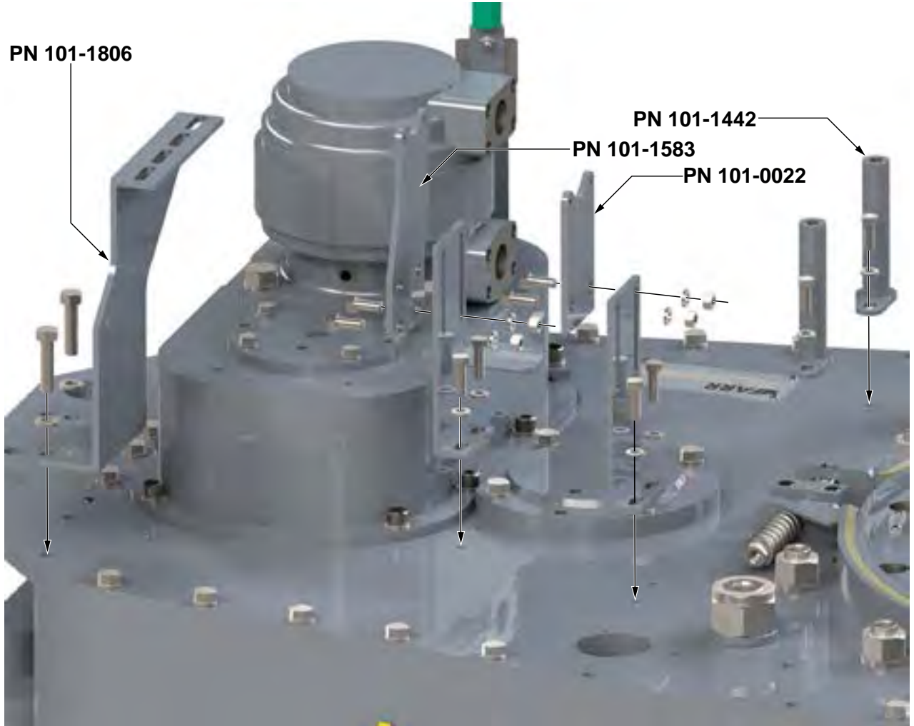
ILLUSTRATION 4.1.17: HYDRAULIC SUPPORT INSTALLATIONS
