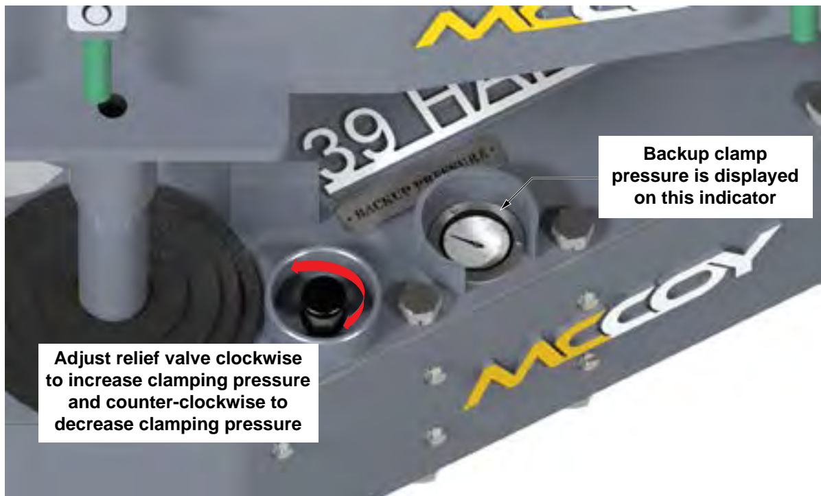
ILLUSTRATION 2.G.7: BACKUP CLAMP PRESSURE ADJUSTMENT
