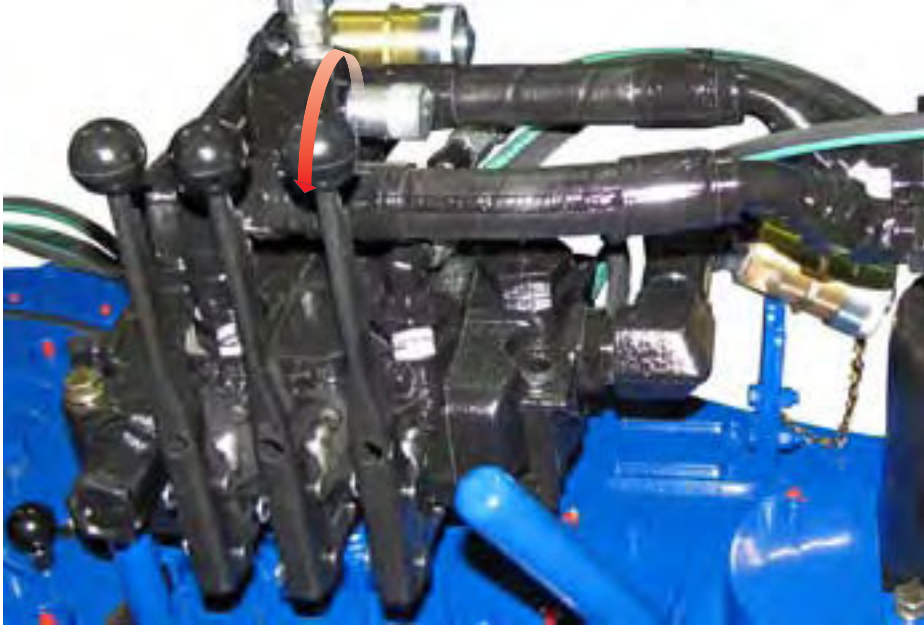
ILLUSTRATION 2.J.10: USING BACKUP CONTROL TO RELEASE BACKUP JAWS
