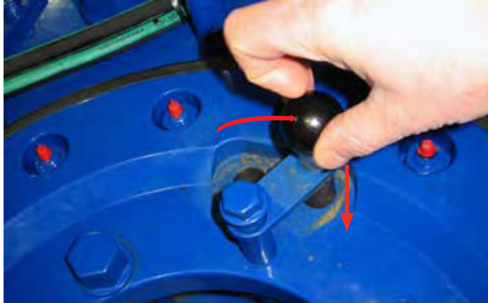
ILLUSTRATION 2.J.12: SETTING BACKING PIN TO BREAK-OUT POSITION
