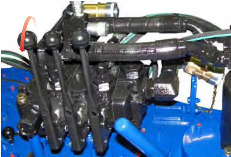
ILLUSTRATION 2.J.9: USING MOTOR CONTROL TO RELEASE JAWS IN "MAKE UP" MODE
