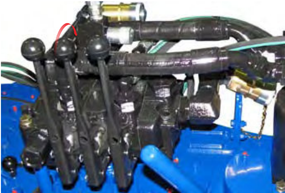
ILLUSTRATION 2.J.11: USING LIFT CYLINDER CONTROL TO LOWER ASSEMBLY (NON CE-MARKED TONGS ONLY)
