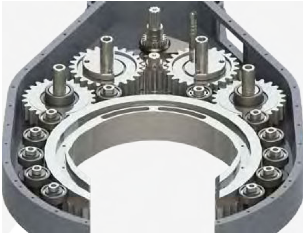
ILLUSTRATION 3.1.2: TONG ASSEMBLY - GEAR ASSEMBLY POSITIONING
