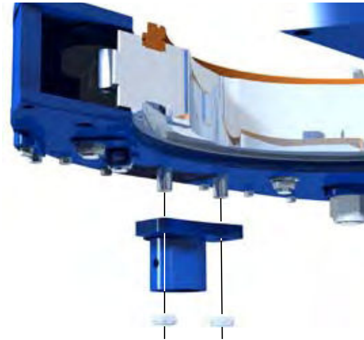
ILLUSTRATION 3.1.8: TONG ASSEMBLY - FRONT LEG MOUNT WELDMENT INSTALLATION
