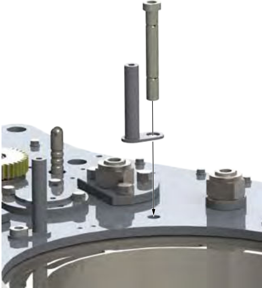
ILLUSTRATION 3.1.5: TONG ASSEMBLY - SUPPORT ROLLER INSTALLATION 02
