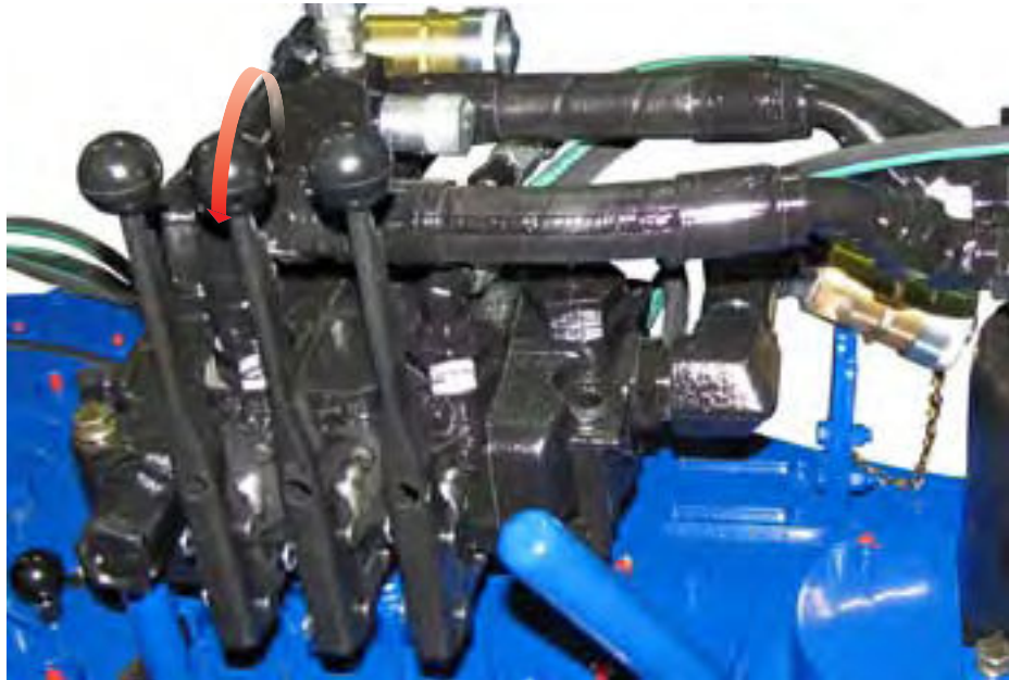
ILLUSTRATION 2.J.6: LIFT CYLINDER CONTROL - RAISE (NON CE-MARKED TONGS)
