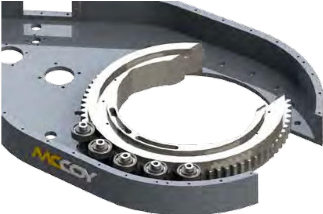
ILLUSTRATION 3.1.1: TONG ASSEMBLY - ROTARY GEAR INSTALLATION
