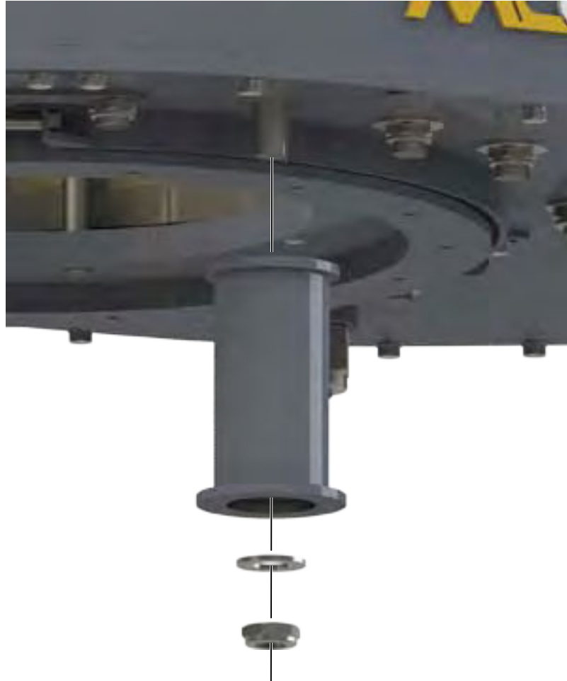
ILLUSTRATION 3.I.8: TONG ASSEMBLY - FRONT LEG INSTALLATION
