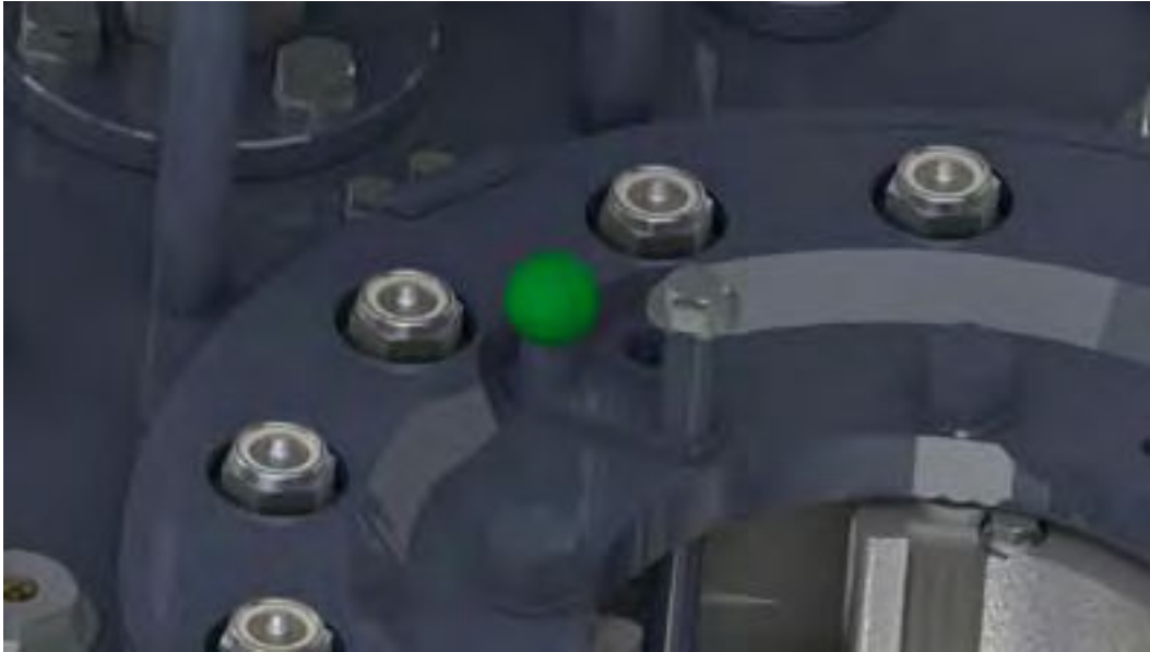
ILLUSTRATION 2.J.2: BACKING PIN SET TO "MAKE-UP" POSITION
