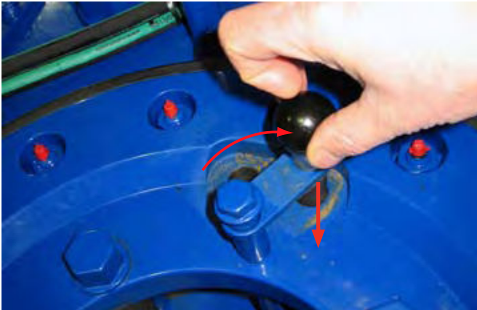
ILLUSTRATION 2.J.8: SETTING BACKING PIN TO "BREAK-OUT" POSITION
