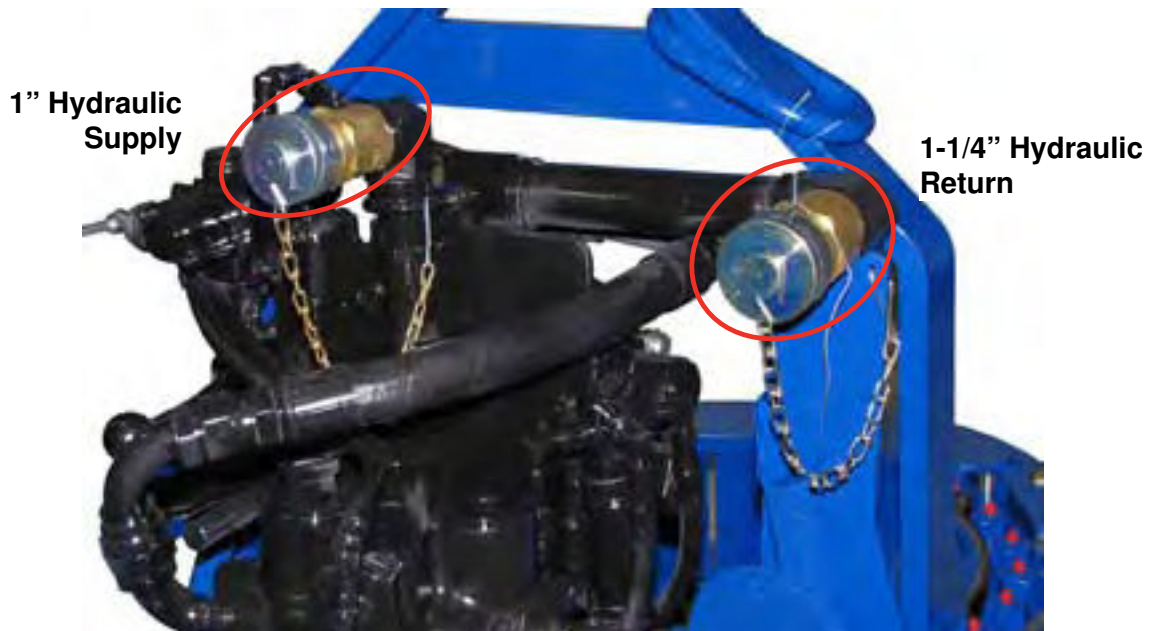
ILLUSTRATION 2.E.7: HYDRAULIC CONNECTIONS 01
