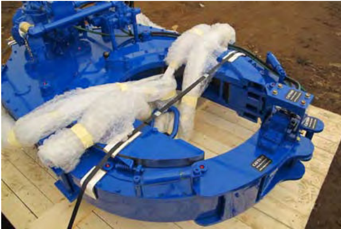
ILLUSTRATION 4.L.2: SHIPPING INSTRUCTIONS - WRAPPING CHAIN SLING
