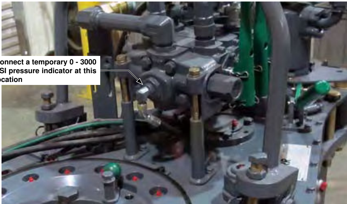
ILLUSTRATION 5.B.1: RELIEF VALVE TROUBLESHOOTING - TEMPORARY GAUGE INSTALLATION
