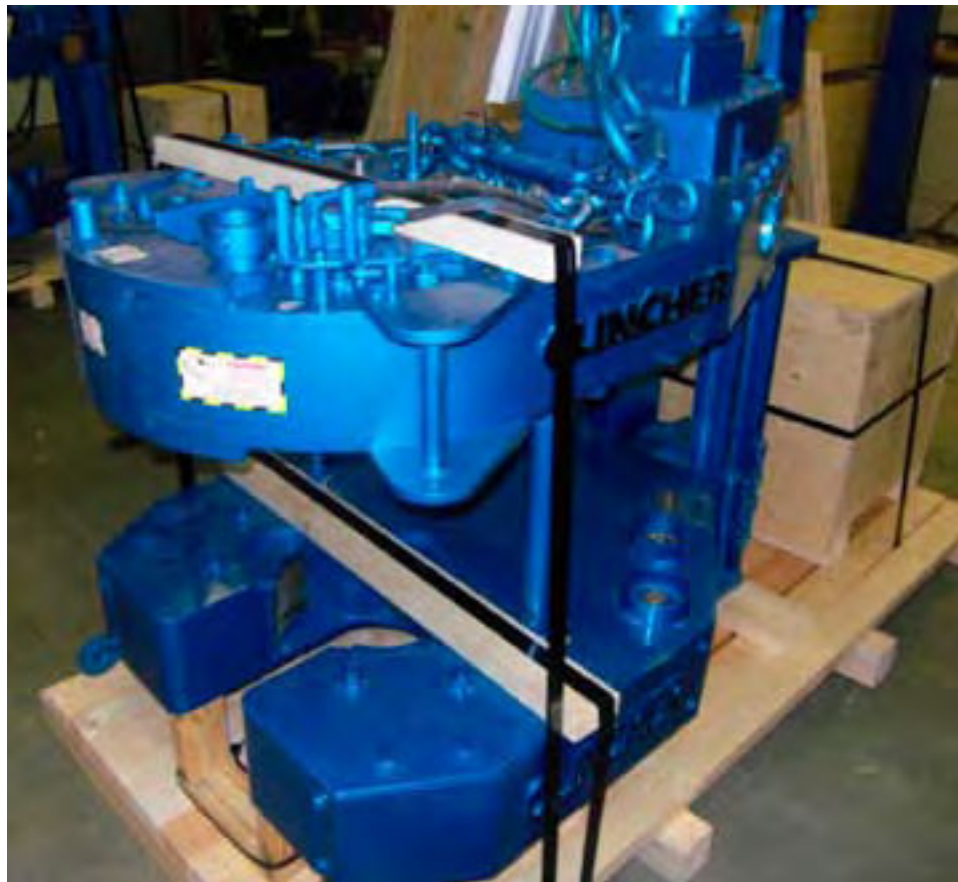
ILLUSTRATION 4.L.4: SHIPPING INSTRUCTIONS - STRAPPING EQUIPMENT TO PALLET
