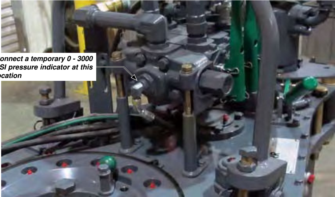
ILLUSTRATION 4.B.1: RELIEF VALVE TROUBLESHOOTING - TEMPORARY GAUGE INSTALLATION
