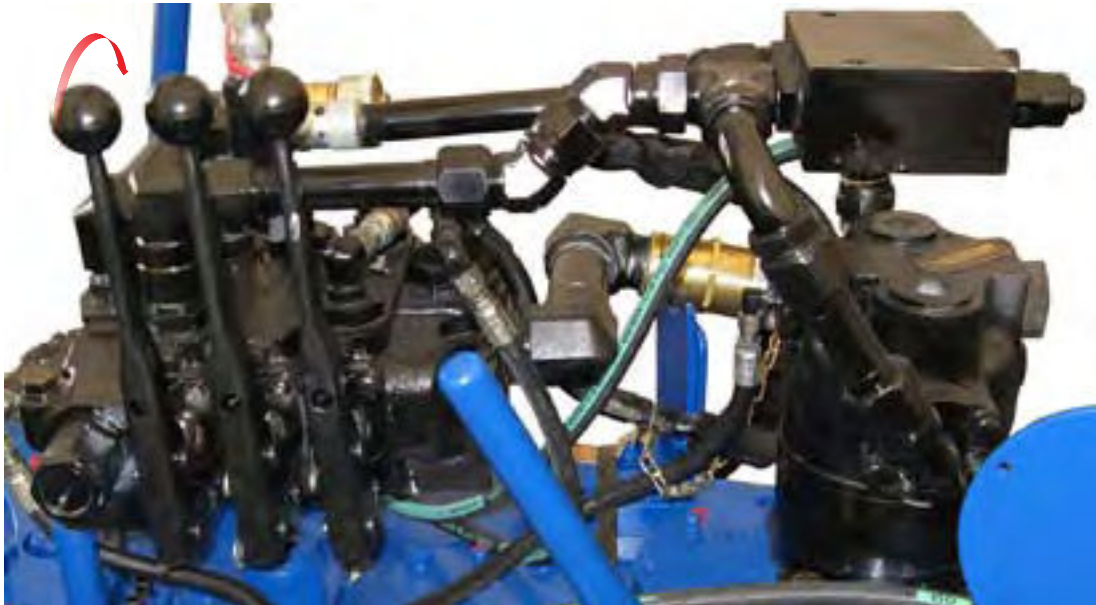
ILLUSTRATION 2.H.12: USING MOTOR CONTROL TO RELEASE TONG JAWS FOLLOWING BREAK-OUT & UN-THREADING
