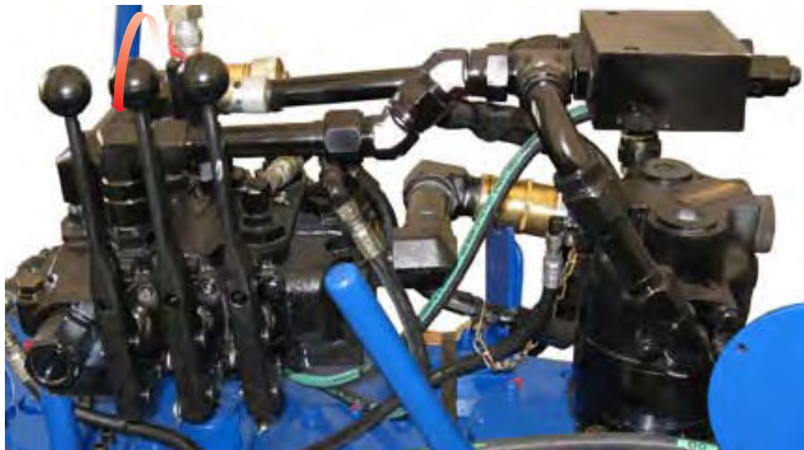
ILLUSTRATION 2.H.13: LOWERING TONG & BACKUP USING LIFT CYLINDER CONTROL
