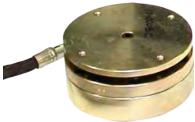
ILLUSTRATION 6.A.3: COMPRESSION LOAD CELL
