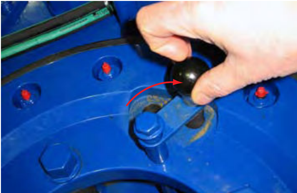
ILLUSTRATION 2.J.8: SETTING BACKING PIN TO "BREAK-OUT" POSITION
