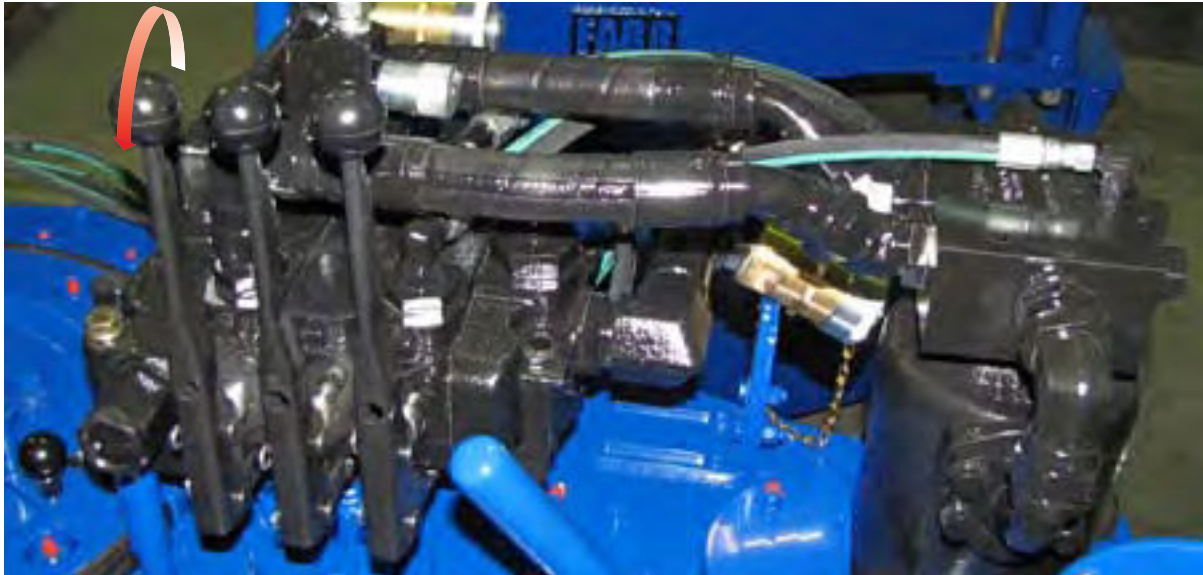
ILLUSTRATION 2.J.9: ROTATION CONTROL - BREAK-OUT
