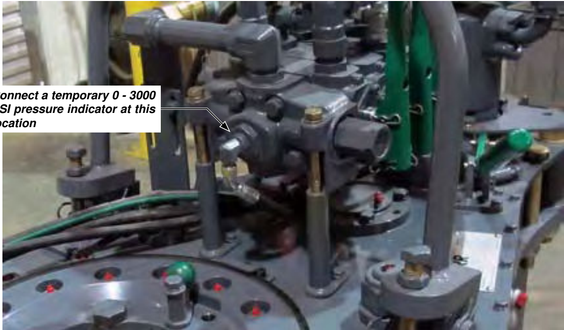
ILLUSTRATION 4.B.1: RELIEF VALVE TROUBLESHOOTING - INSTALLING TEMPORARY PRESSURE GAUGE
