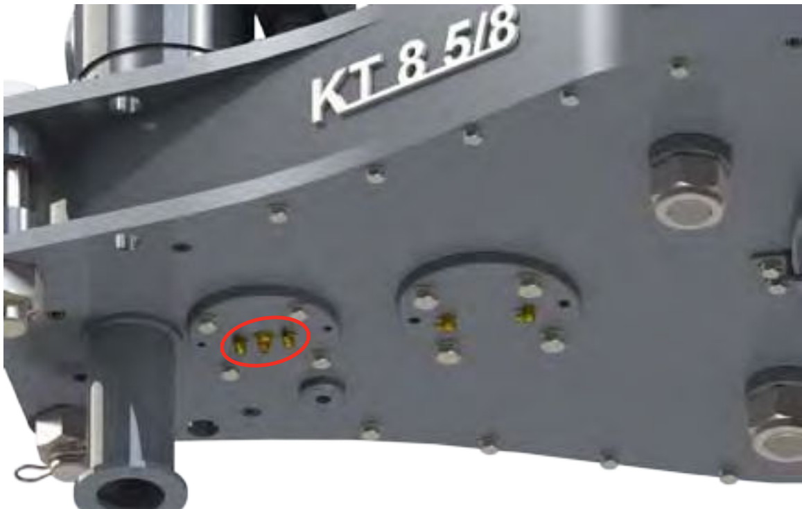
ILLUSTRATION 3.E.7: CLUTCH LUBRICATION POINTS
