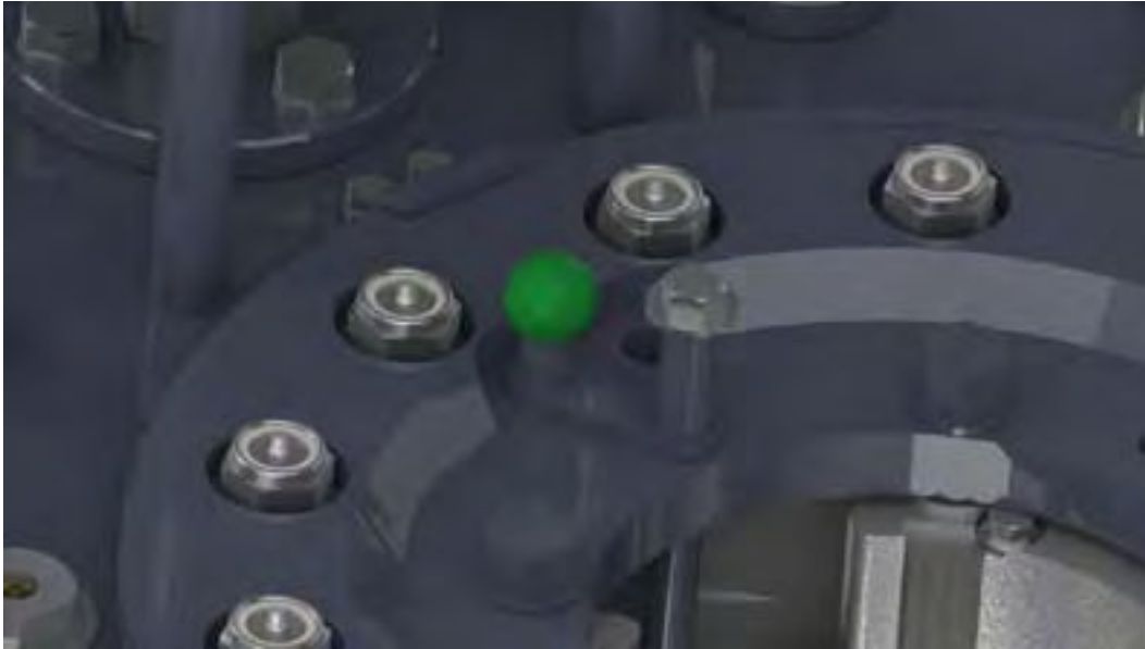
ILLUSTRATION 2.J.2: BACKING PIN SET TO "MAKE-UP" POSITION
