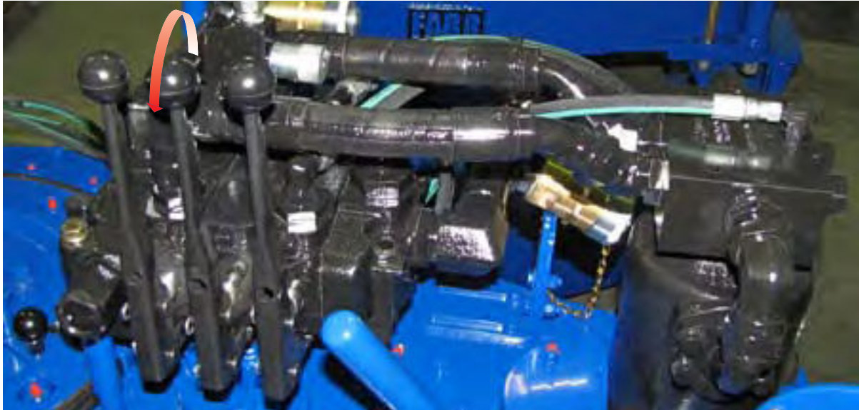
ILLUSTRATION 2.J.3: LIFT CYLINDER CONTROL - RAISE
