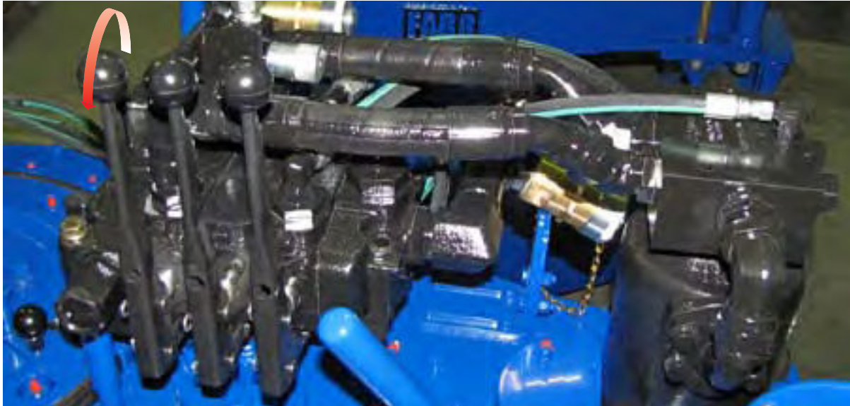
ILLUSTRATION 2.J.6: MOTOR CONTROL - RELEASING JAWS
