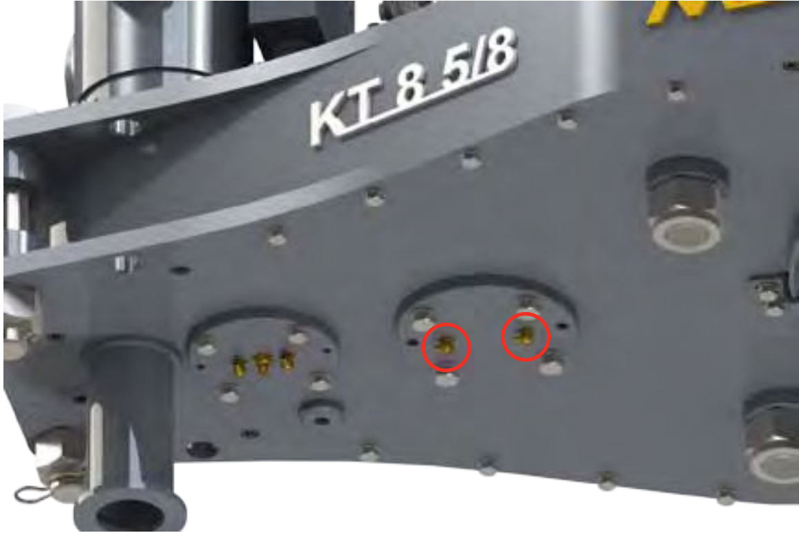
ILLUSTRATION 3.E.6: PINION LUBRICATION POINTS (BOTTOM PLATE)
