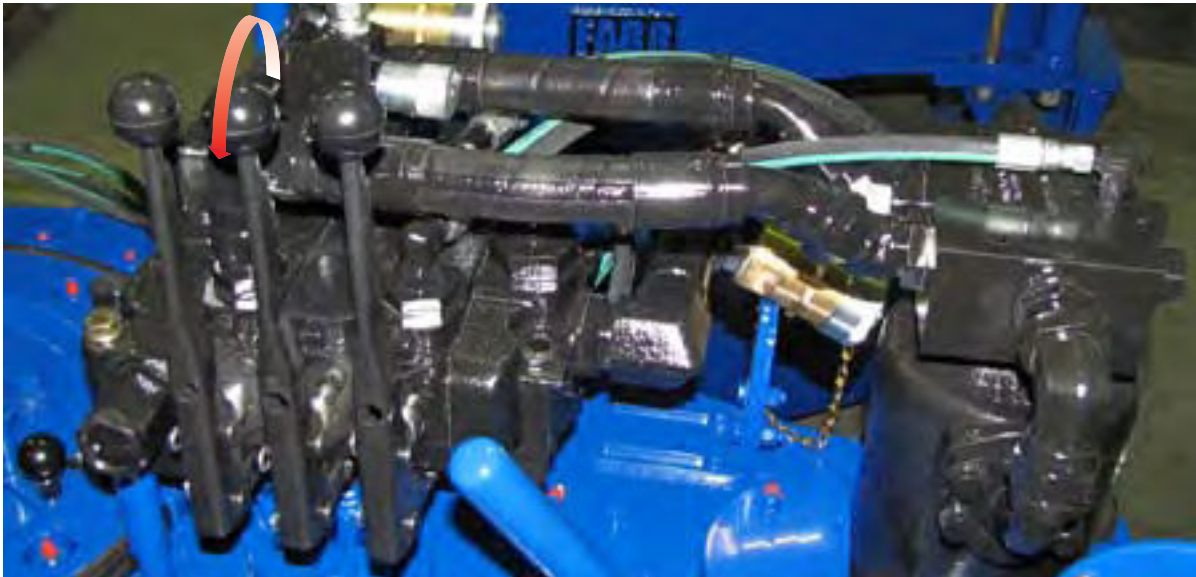
ILLUSTRATION 2.J.11: LOWERING TONG USING LIFT CYLINDER CONTROL
