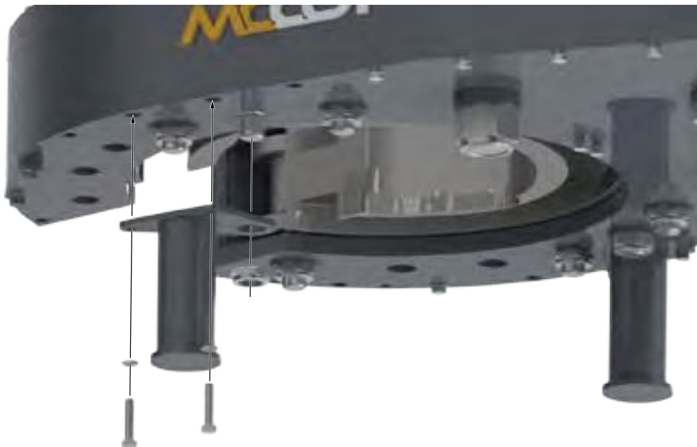
ILLUSTRATION 3.I.5: TONG ASSEMBLY - FRONT LEG INSTALLATION
