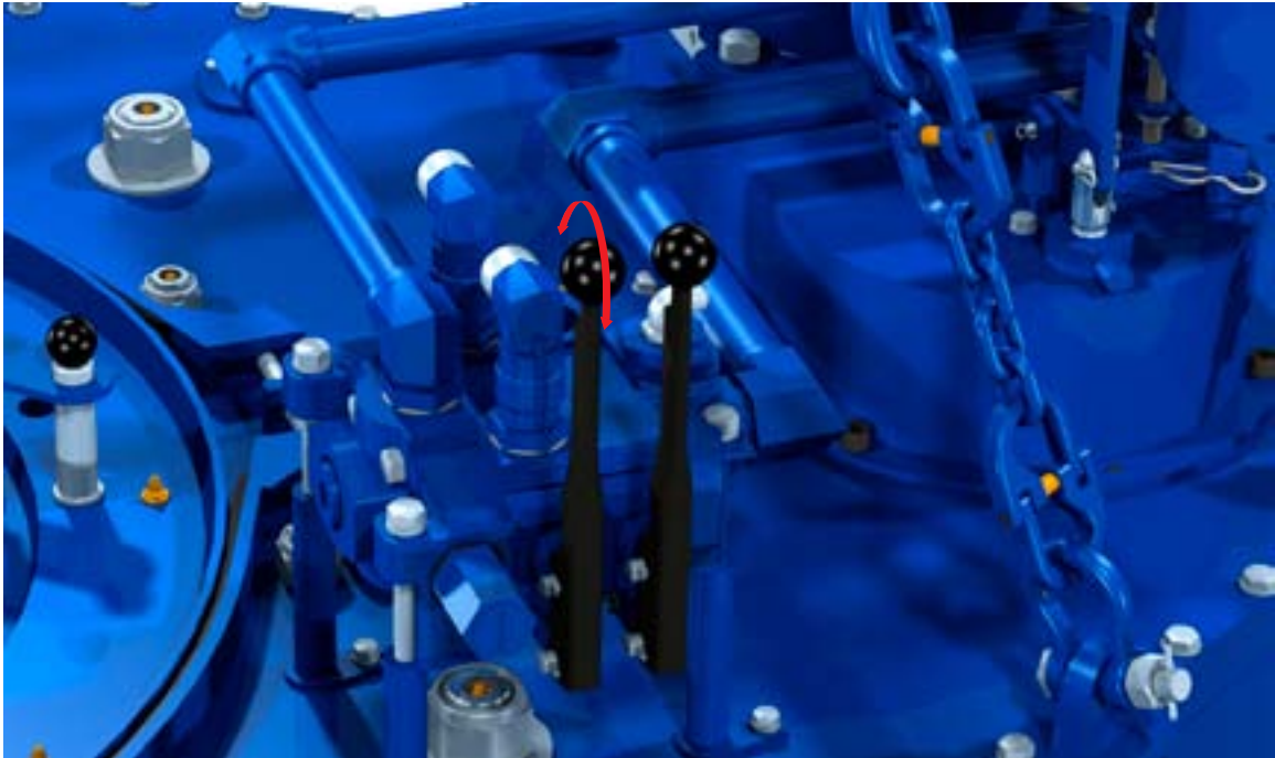
ILLUSTRATION 2.G.1: TONG ROTATION CONTROL VALVE
