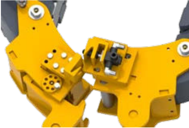
Incorrect engagement at one floating plate extreme position (switch impacts and binds on fixed safety door components)
