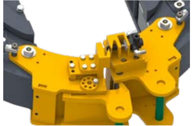
Incorrect engagement at second floating plate extreme position (claws do not engage).
