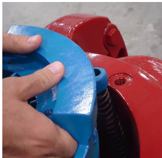
Figure 3 – Compressing spring to install slip
