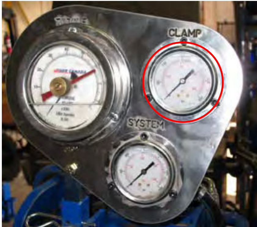
ILLUSTRATION 2.1.4: CLAMP PRESSURE GAUGE ON GAUGE PANEL
