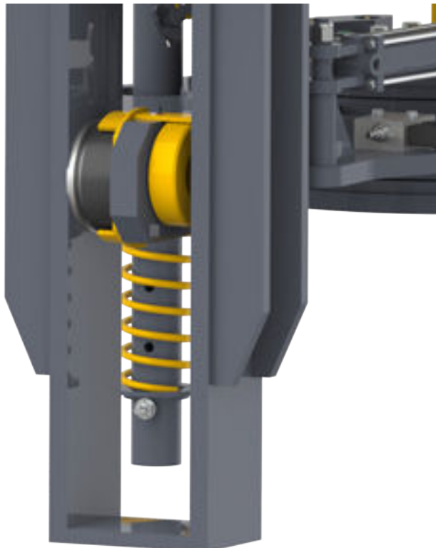
Load cell configured for make-up operations
