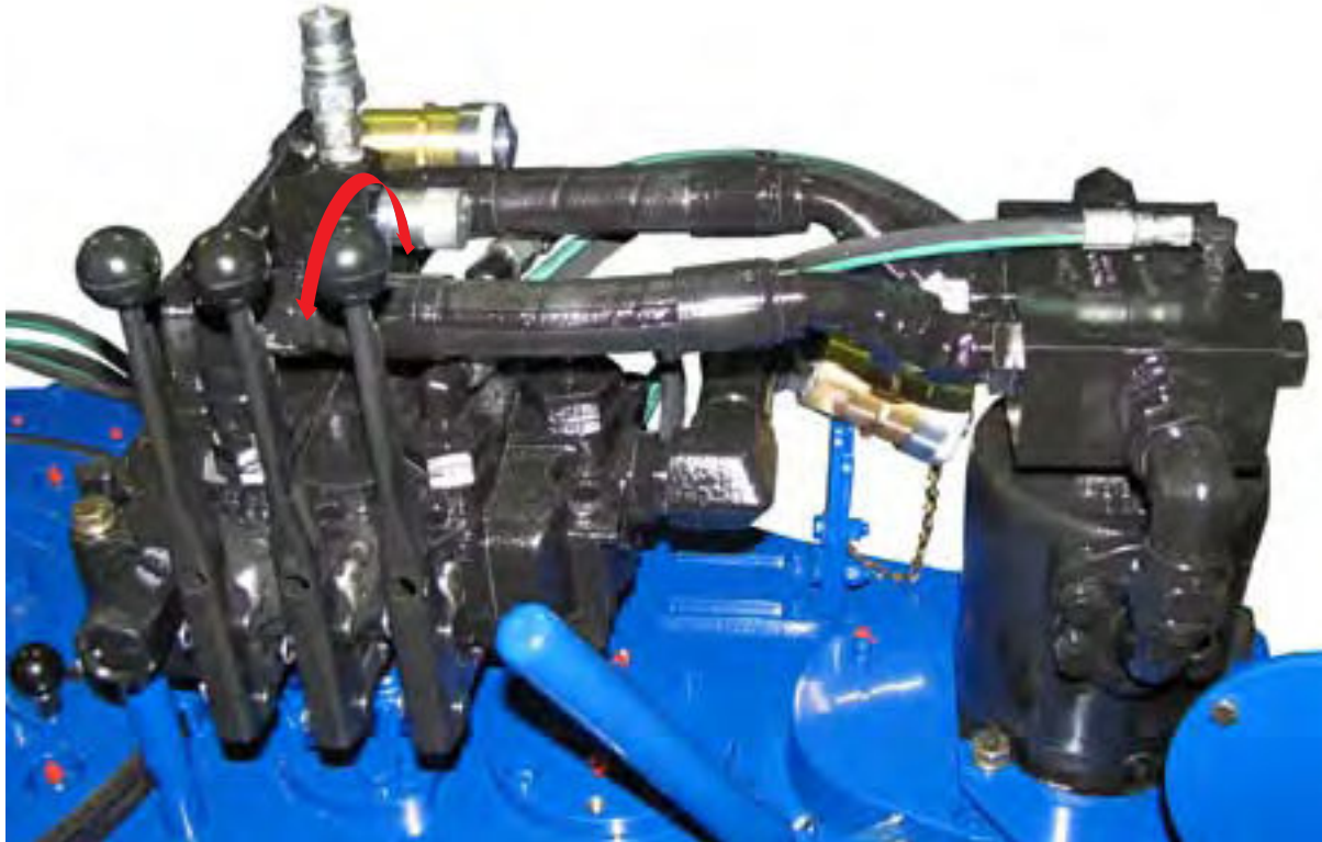
ILLUSTRATION 2.G.1: HYDRAULIC CONTROL - BACKUP
